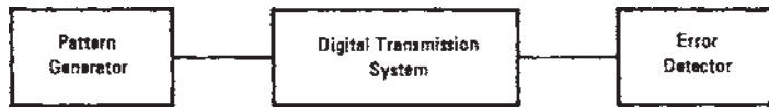
Figure 31.3 To test a digital transmission system, a pattern generator is connected to the input of the system under test, and an error detector is connected at the output.
