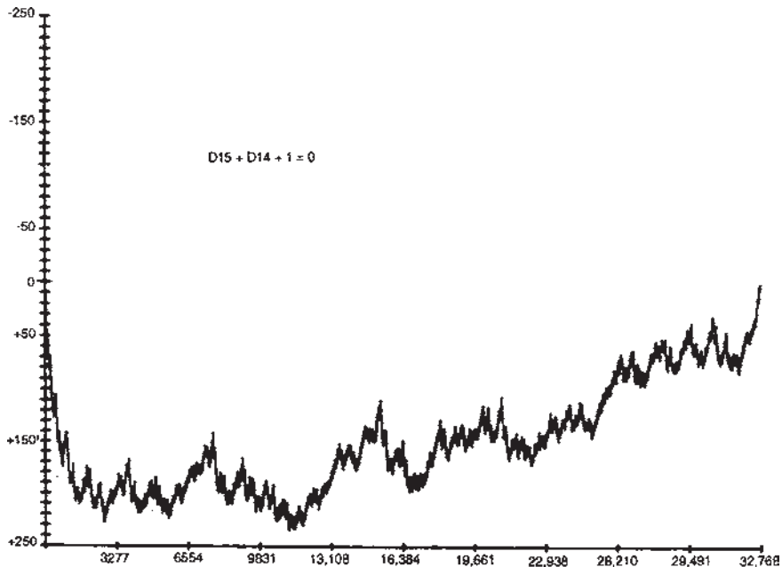
Figure 31.8 This graph shows the running digital sum for a commonly used PRBS. Notice the initial steep descent of the graph, indicating a predominance of ones or zeros (depending on inversion) for the initial period of the sequence.
