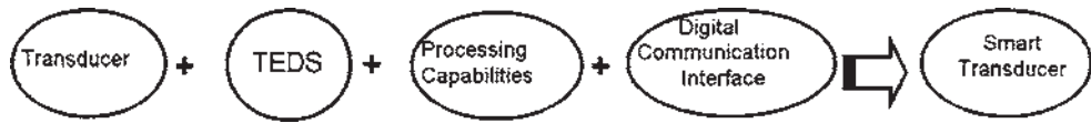
Figure 47.9 A transducer can be either a sensor or actuator. A smart transducer is a transducer integrated with a TEDS, has microprocessing capability to perform some intelligent functions, and has a digital communication interface for outputting (Per IEEE 1451.2).
