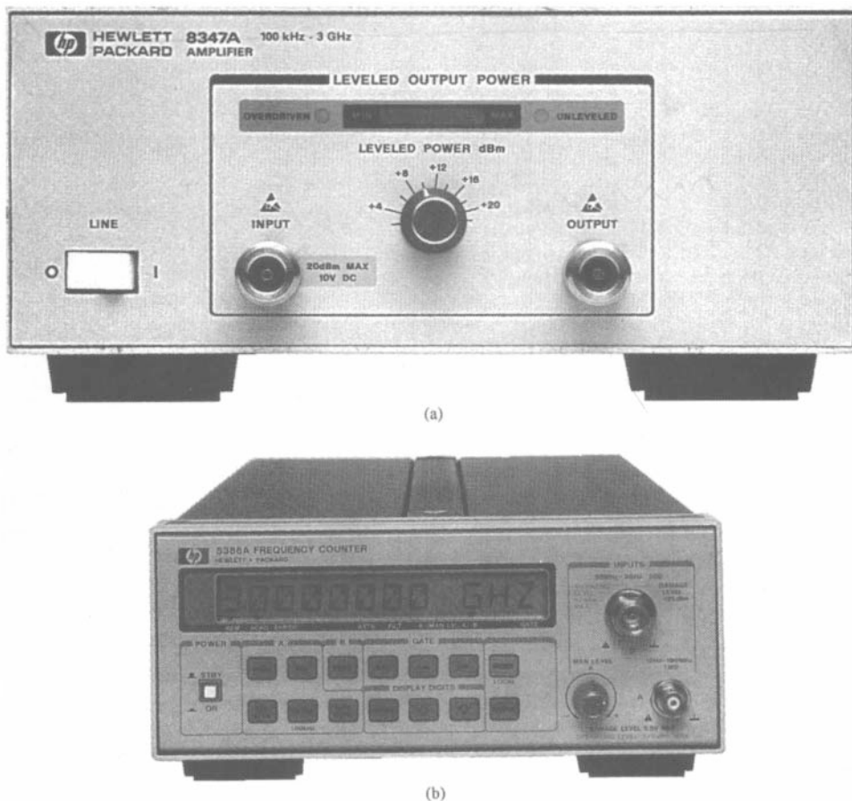
Figure 12.2 Three display types and technologies commonly found in instruments. (a) Indicator lights. (b) Small alphanumeric display implemented with liquid-crystal display (LCD) technology. (c) Small alphanumeric displays implemented with light-emitting diode (LED) display technology. (d) Graphics and text display implemented with cathode-ray tube (CRT) display technology.
