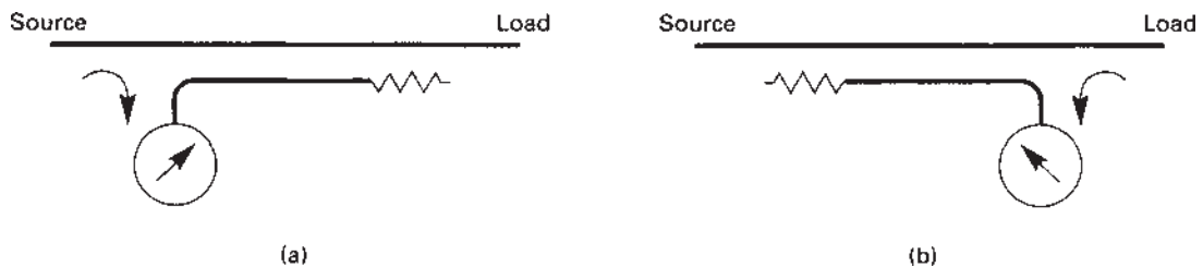
Figure 15.4 Transmission-type rf power meters respond to the direction and magnitude of power flow. (a) Measure power flow from source to load; (b) measure power flow from load to source.
