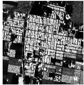
Buildings are very bright in a radar image of a town because the building sides act as corner reflectors.
