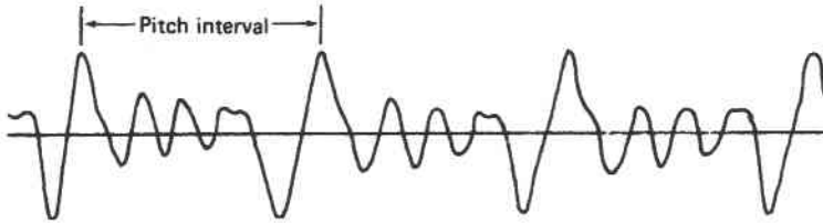
Figure 3.23 Time waveform of voiced sound.
