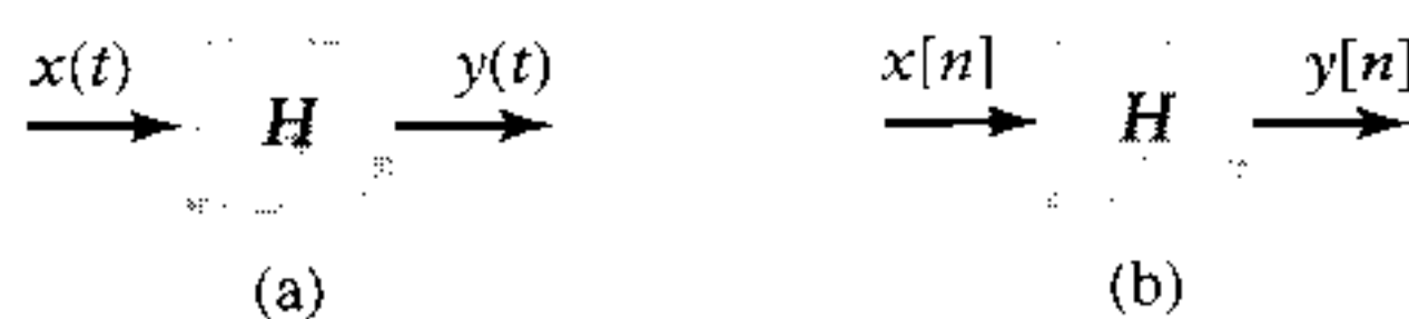
FIGURE 1.43 Block diagram representation of operator H for (a) continuous time and (b) discrete time.
