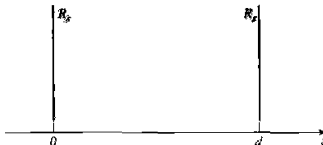
FIGURE 6.13 An idealized Fabry-Perot resonator consisting of two parallel conducting plates.
