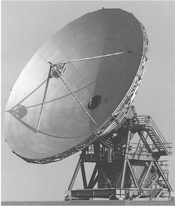
Figure 6.22 A 19-m Cassegrain antenna. (Courtesy of TIW Systems, Inc.)
