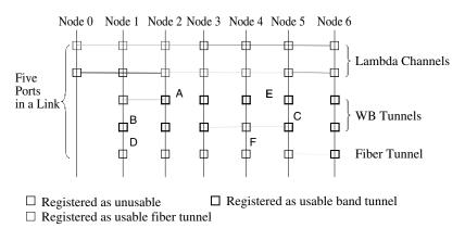
Figure 11.5 An example of dynamic tunnel allocation. (P.H. Ho and H.T. Mouftah, Routing and wavelength assignment with multi-granularity traffic in optical networks, IEEE, Aug. 2002. With permission.)
