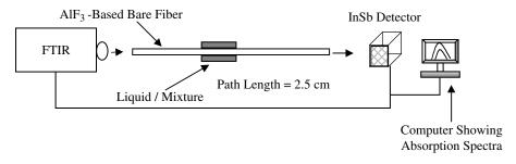
*Figure 20.17* Experimental setup for the detection of chemical species by evanescent absorption of fundamental modes by using AIF<sub>3</sub>-based fibers.
