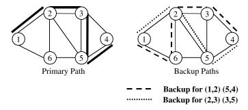
Figure 17.2 Backup path assignment using PPP.
