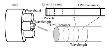
*Figure 11.1* Illustration of the traffic hierarchy defined in GMPLS. (P.H. Ho and H.T. Mouftah, Routing and wavelength assignment with multi-granularity traffic in optical networks, IEEE, Aug. 2002. With permission.)
