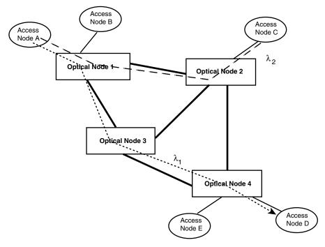
*Figure 12.1* A wavelength-routed optical WDM network including optical switching nodes and access nodes. Lightpaths are established between pairs of access nodes on different wavelengths.
