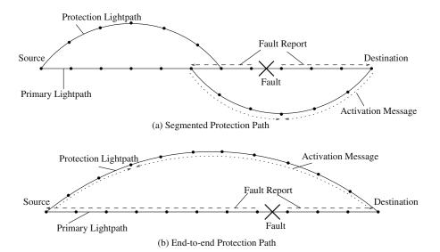
*Figure 16.7* Illustration of failure recovery.
