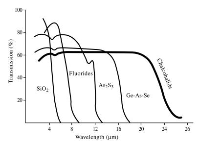
Figure 20.6 Transmission spectra of various glass systems.
