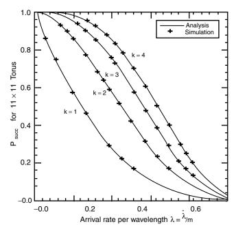
*Figure 12.7* Analytical and simulation results for  $P_{succ}$  vs. the arrival rate per wavelength  $\lambda = \lambda / k$ , for an 11 × 11 torus network, using oblivious XY routing.
