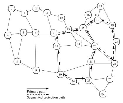
Figure 16.4 No end-to-end protection path but segmented protection path exists.
