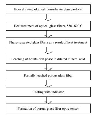
Figure 20.26 Flow chart for the production of porous fiber optic sensors.
