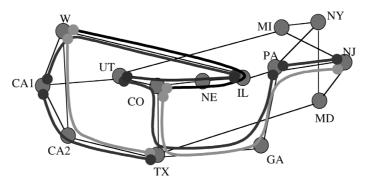
Figure 1.8 Lightpath connections in a WDM mesh network. (Solid circles mark the end points of a lightpath.)
