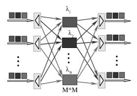
*Figure 1.5* An optical crossconnect (OXC) of size NM x NM (N is the number of wavelengths; M is the number of incoming/outgoing fibers).
