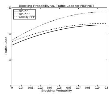
Figure 17.3 Traffic load vs. blocking probability: NSFNET.
