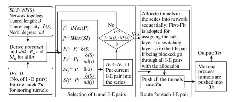
Figure 11.7 Flowchart for summarizing the algorithm of the static tunnel allocation as a strategy of network planning. Assume that the network has N nodes. We define  $iMax(Q_i)$ , which returns the indexes I, such that  $Q_I = \max(Q_i)$ . IE is an index to count the number of tunnels in the series. (P.H. Ho and  $H^{\tilde{I}}$ . Mouftah, Routing and wavelength assignment with multi-granularity traffic in optical networks, IEEE, Aug. 2002. With permission.)
