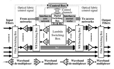
*Figure 11.2* Architecture of a node that implements multi-granularity traffic tunneling. (P.H. Ho and H.T. Mouftah, Routing and wavelength assignment with multi-granularity traffic in optical networks, IEEE, Aug. 2002. With permission.)
