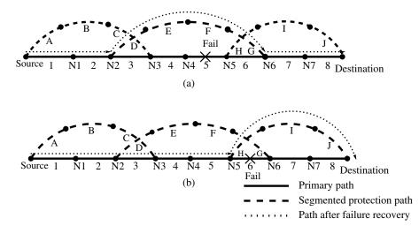
Figure 16.2 Illustration of segmented protection paths.
