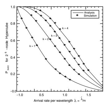
*Figure 12.6* Analytical and simulation results for  $P_{succ}$  vs. the arrival rate per wavelength  $\lambda = \hat{\lambda}/k$ , for a 2<sup>6</sup>-node hypercube network, using oblivious routing.
