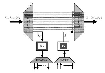
Figure 19.7 Subrate multiplexing makes efficient use of wavelength bandwidth by aggregating/grouping data at OADM nodes.
