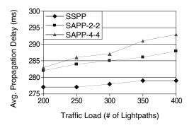
*Figure 18.8* Impacts of traffic changes and protection schemes on the average propagation delay of primary lightpaths.
