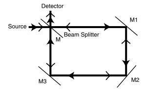
Figure 21.3 Classical sagnac interferometer.
