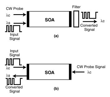
*Figure 21.5* XGM wavelength conversion principle: (a) co-propagating signals; (b) counter-propagating signals.
