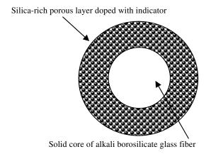
Figure 20.27 Cross section of porous glass fiber.
