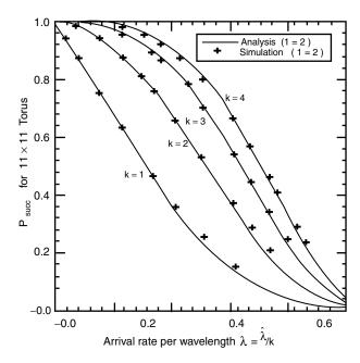
*Figure 12.8* Analytical and simulation results for  $P_{succ}$  vs. the arrival rate per wavelength for an 11 × 11 torus hypercube network, using adaptive VCD routing.
