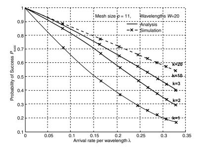
*Figure 12.3* Success probability  $P_{succ}$  vs. the arrival rate per wavelength  $\lambda$ , for a  $p \times p$  torus (p = 11), for W = 20 wavelengths per link.
