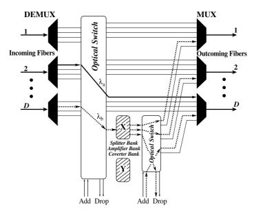
*Figure 1.13* Transparent OXC architecture for supporting multicasting using optical splitters.
