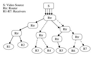
Figure 7.1 Replicated video multicast using DSG protocol.
