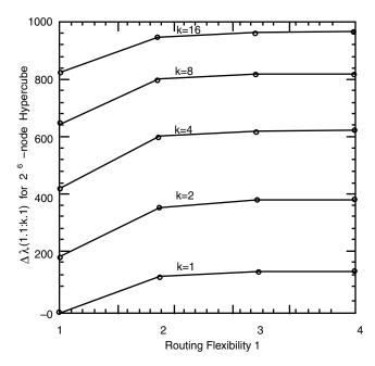
*Figure 12.12* The incremental throughput gain  $\lambda(1, 1; k, l)$ , for k = 1, 2, 4, 8, 16 and l = 1, 2, 3, 4, for a 2<sup>6</sup>-node hypercube network with  $P_{succ} = 0.8$ .
