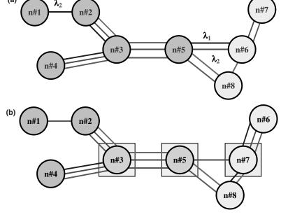
*Figure 19.8* (a) Due to wavelength continuity constraints, certain traffic (e.g.,  $\lambda_1$ ,  $\lambda_2$ ) (blue, green) is unroutable through certain nodes (no. 3 and no. 5) because those wavelengths are in use. (b) Wavelength conversion allows transparency throughout the network.
