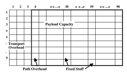
Figure 19.1 Structure of basic SONET frame, a  $9 \times 90$  matrix with 84 data columns (i.e., 756 bytes for payload [48.384 Mb/s]).
