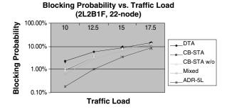
Figure 11.11 Blocking probability vs. traffic load with different percentages of switching types in the 16-node and 22-node networks. CB-STA w/o is a CB-STA tunnel allocation without the makeup process. (continued)
