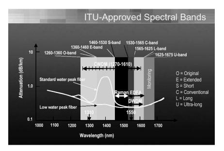
*Figure 19.3* ITU-T-approved band assignment in the low attenuation window of the silica fibers; the wavelength range involves 1260–1360 nm = O-band; 1360–1460 nm = E-band; 1460–1530 nm = S-band; 1530–1565 nm = C-band; 1565–1625 nm = L-band; and 1625–1675 nm = U-band (used in monitoring). (Courtesy EXFO Electro-Optical Engineering Inc. Printed with permission.)
