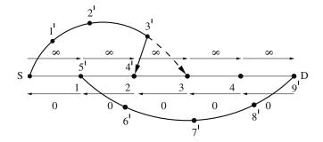
Figure 16.6 Illustration of the construction of modified graph G' and the shortest segmented protection path from the path chosen.
