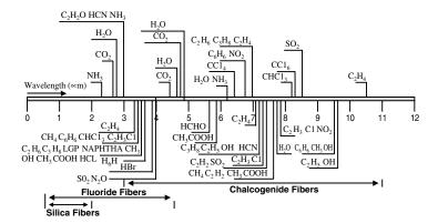
*Figure 20.16* IR signatures of food products, fertilizers, drugs, plastics, petrochemicals, and gases, as well as the transmission range of various fibers.
