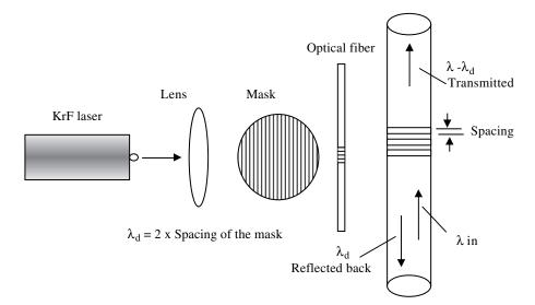
Figure 20.9 Experimental setup for making fiber gratings.
