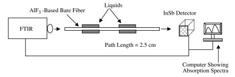
*Figure* 20.20 Experimental setup for a wavelenth-division-multiplexed distributed fiber optic chemical sensor for simultaneous detection of a variety of chemical species.
