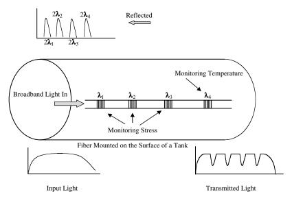
Figure 20.12 Wavelength-division-multiplexed fiber-optic Bragg grating sensor for simultaneous detection of stress and temperature.
