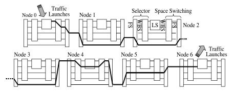
*Figure 11.3* Switching process of a lightpath that is sourced at node 0 and destined at node 6. (P.H. Ho and H.T. Mouftah, Routing and wavelength assignment with multi-granularity traffic in optical networks, IEEE, Aug. 2002. With permission.)
