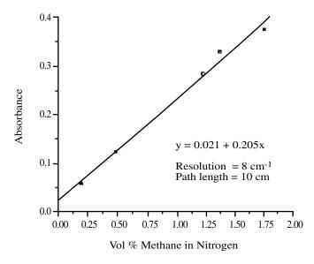
*Figure* 20.25 Calibration curve for methane in nitrogen. (From S.J. Saggese et al., *SPIE Proc.*, 1172, 2, 1990. With permission.)
