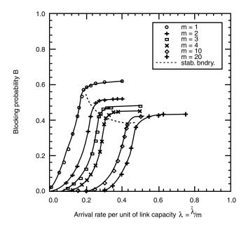
*Figure 12.4* Performance results for the VCD protocol, illustrating the blocking probability B as a function of the normalized arrival rate per unit of link capacity  $\hat{\lambda}/m$  for an  $8 \times 8$  MS network and several values of m. The dashed lines correspond to the stability boundary.
