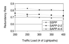
Figure 18.9 Impacts of traffic changes and protection schemes on the network redundancy rate.
