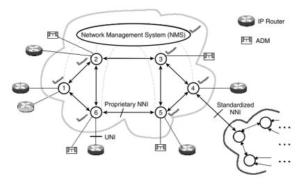
Figure 1.15 Network management system for IP-over-WDM networks.
