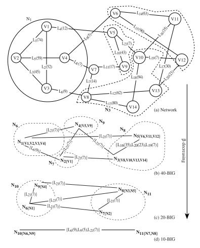
Figure 9.9 The blocking island hierarchy for bandwidth requirement {40, 20, 10}: (a) the network graph; (b) the 40-BIG; (c) the 20-BIG; (d) the 10-BIG.
