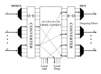
Figure 1.12 Opaque OXC architecture for supporting multicasting using electronic crossconnect.
