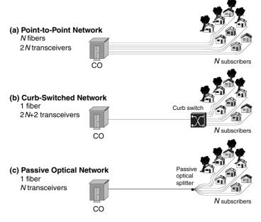
Figure 1.6 Different technologies for fiber-to-the-home (FTTH).
