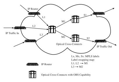
Figure 9.7 An IP-over-OBS WDM transmission backbone using MLPS.
