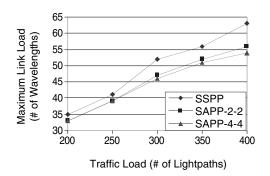
Figure 18.10 Impacts of traffic changes and protection schemes on the maximum link load.
