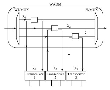
Figure 9.1 WADM structure. Three wavelengths, 1, 2, 2, are in the fiber.
