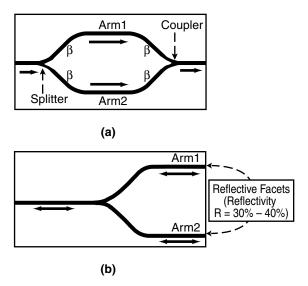
Figure 21.2 (a) Mach–Zehnder interferometer; (b) Michelson interferometer.
