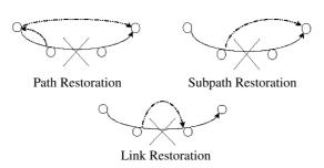
Figure 1.10 Mechanisms for restoring connections after fiber failure.
