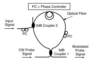
Figure 21.4 Nonlinear-optical loop mirror using optical fiber.
