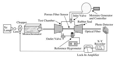
Figure 20.28 Schematic diagram of experimental setup for porous glass fiber optic humidity sensor.
