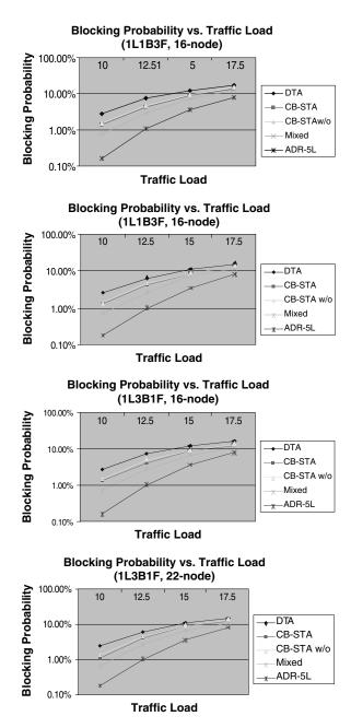
*Figure 11.11 (continued)* Blocking probability vs. traffic load with different percentages of switching types in the 16-node and 22-node networks. CB-STA w/o is a CB-STA tunnel allocation without the makeup process. (P.H. Ho and H.T. Mouftah, Routing and wavelength assignment with multi-granularity traffic in optical networks, IEEE, Aug. 2002. With permission.)
