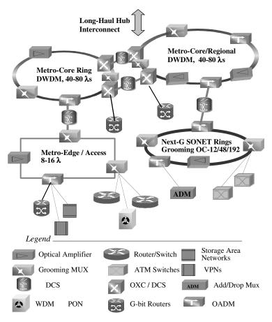
Figure 2.5 Metro optical networks architecture from edge-to-core.
