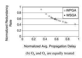
*Figure 18.7* Pareto-optimal front and best solution obtained from WPGA and WSGA, respectively, after 500 generations.
