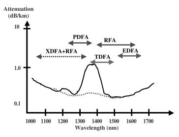
*Figure 19.5* Shows the typical loss dB/km of single-mode fiber (silica) as a function of wavelength and a variety of optical amplifiers covering the low-loss region that constitutes the transmission window, which is subdivided into multiple bands. Rare-earth doped fiber amplifiers (XDFA) and Raman fiber amplifiers (RFA) provide gain over the entire 400 nm low attenuation window.
