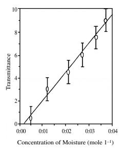
*Figure* 20.30 The calibration curve for the porous glass fiber optic moisture sensor doped with 0.03 b/ml hydrated cobalt (II) sulphate at the temperature of 160°C. (From J.Y. Ding et al., *Int. J. Optoelect.*, 6, 385, 1991. With permission.)
