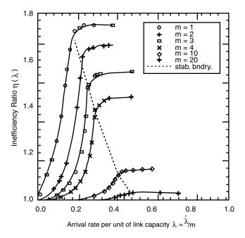
*Figure* **12.5** Performance results for the VCD protocol, illustrating the inefficiency ratio  $\eta(\lambda)$  as a function of the normalized arrival rate per unit of link capacity  $\lambda = \hat{\lambda}/m$ , for an 8 × 8 MS network and several values of m. The dashed lines correspond to the stability boundary.
