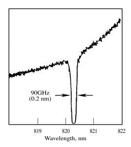
*Figure 20.10* Typical fiber grating transmission spectrum. (From W.W. Morey et al., *SPIE Proc.*, 1586, 1, 1991. With permission.)
