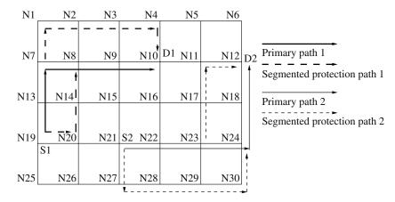
*Figure 16.5* Segmented protection paths are more flexible for routing than end-to-end protection paths.
