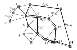
*Figure 11.4* An example for deriving the weighted network link state (W-NLS) for the link *i-j.* (P.H. Ho and H.T. Mouftah, Routing and wavelength assignment with multi-granularity traffic in optical networks, IEEE, Aug. 2002. With permission.)
