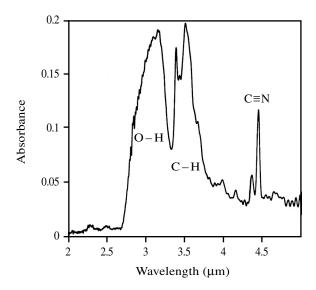
*Figure 20.21* Remote absorption spectra of alcohol and acetonitrile taken by a wavelenth-division-multiplexed distributed AIF<sub>3</sub>-based fiber-optic chemical sensor. (From T. Iqbal et al., *Optics Lett.*, 16, 1611, 1991. With permission.)
