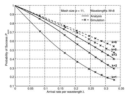
*Figure 12.2* Success probability  $P_{succ}$  vs. the arrival rate per wavelength  $\lambda$ , for a  $p \times p$  torus (p = 11), for W = 8 wavelengths per link.
