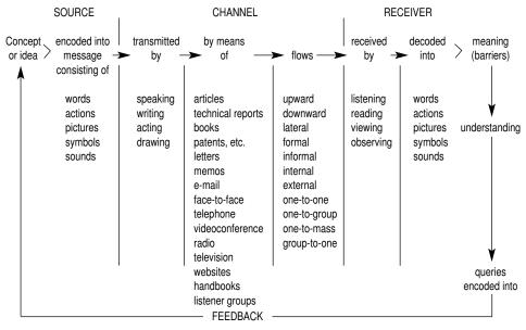
Figure 3.3 Elements of Engineers' Communication
