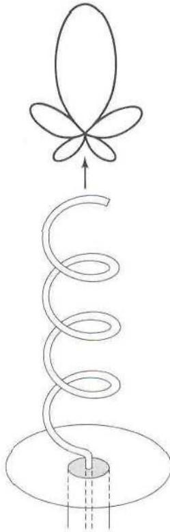
Figure 10.15 Axial (endfire) mode of helix.
