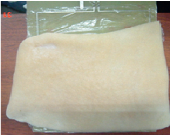
Fig. 7 The inspection of skin using interdigital sensor
