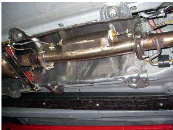
Fig. 21 The UV gas sensor mounted underneath the car
