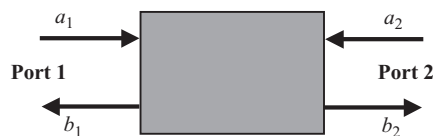
Figure 7.1 A two-port network
