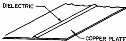
FIG. 42-24 Image line using HE_{11} mode.
