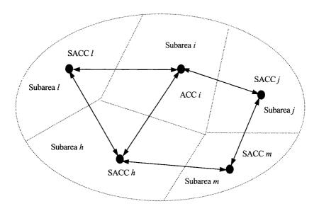
Figure 5.3 System Partitioning for Distributed Load Flow Computation
