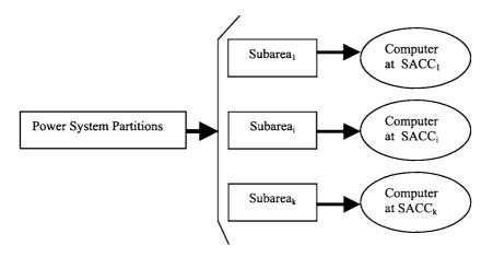
Figure 2.7 Task Allocation for Distributed Load Flow Computation
