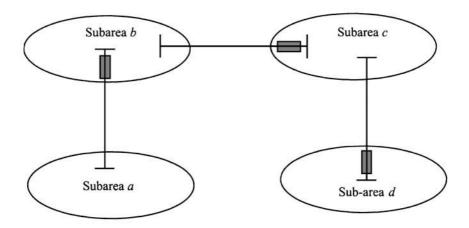
Figure 7.9 Observable System with Fewer Boundary Measurements
