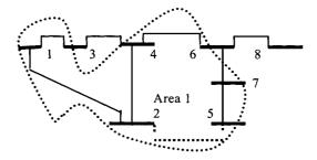
Figure 8.13 First Extension of the Interest Subarea of the Outage of Line 2-5
