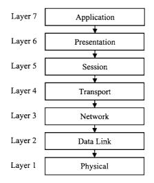
Figure 3.12 OSI Seven-Layer Model
