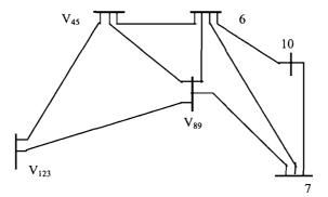
Figure 9.7 System Partitioning Results after Bus 8 and Bus 9 are Merged
