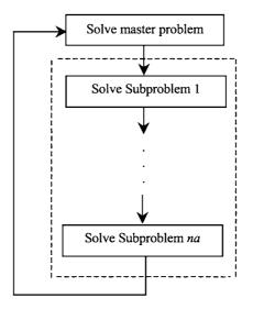
Figure 9.21 Serial Solution of the Dantzig-Wolfe Method
