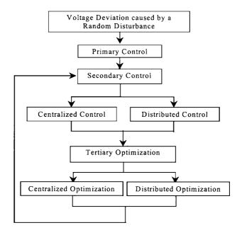
Figure 9.1 Hierarchical and Distributed Voltage/VAR Optimization and Control
