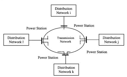
Figure 2.15 Networks of Distribution System
