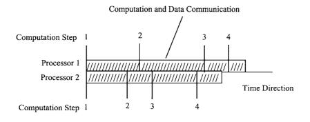
Figure 2.11 Asynchronous Computation
