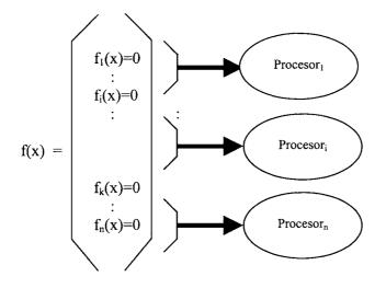
Figure 2.6 Task Allocation for Parallel Load Flow Computation
