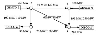
Figure 10.14 Congestion Mitigation with a Standby Transmission Line
