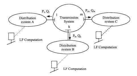
Figure 11.9 Distributed Computation of Load Flow for Distribution System
