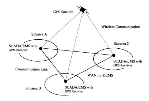
Figure 12.16 GPS for Distributed Processing of DEMS
