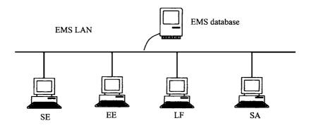
SE: State estimation, EE: External equivalent, LF: Load flow, SA: Security analysis
