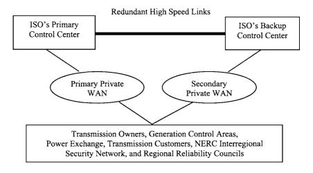
Figure 3.10 Redundant ISO Intranet Configurations
