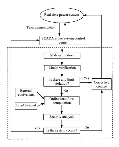
Figure 7.1 Power System State Estimation
