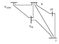
Figure 9.8 System Partition Results after Bus v123 and Bus v45 Are Merged
