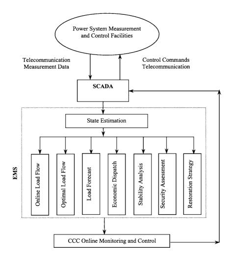
Figure 1.5 Function Structures of SCADA/EMS
