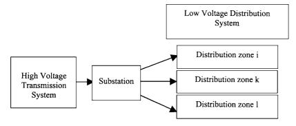
Figure 6.1 Transmission and Distribution Systems
