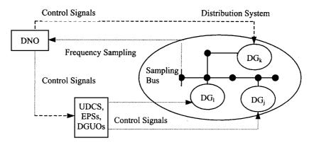
Figure 11.11 Closed-Loop Frequency Control
