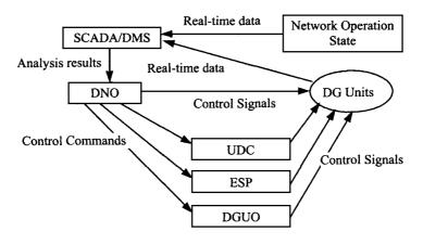
Figure 11.6 Real-Time Monitoring and Control of Distribution System
