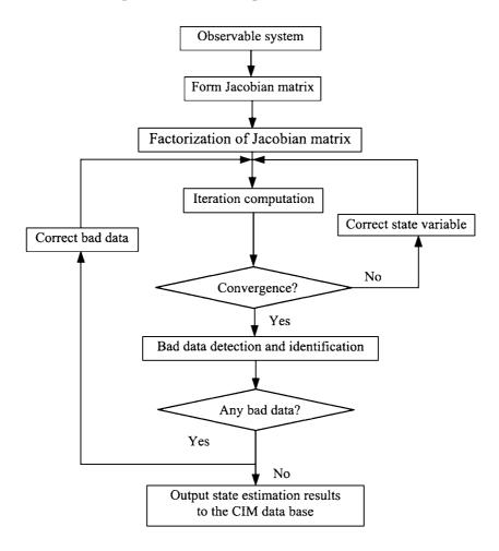
Figure 7.3 Flow Chart of State Estimation
