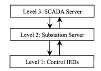
Figure 1.4 Substation Communication Network
