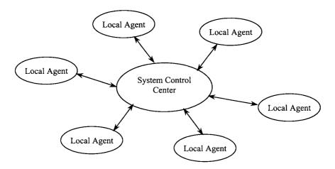
Figure 10. 2 Distributed Control with Autonomous Agents
