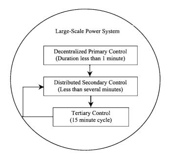
Figure 9.2 Hierarchical and Distributed Voltage/VAR Optimization and Control
