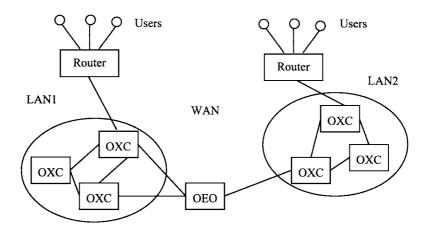
Figure 1.2 Fiber Optical Network
