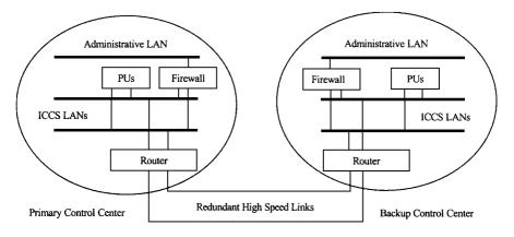
Figure 3.2 Redundant Structure of ICCS
