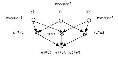
*Figure* 2.5 Parallel Computation of (x1\*x2 + x1\*x3 + x2\*x3)
