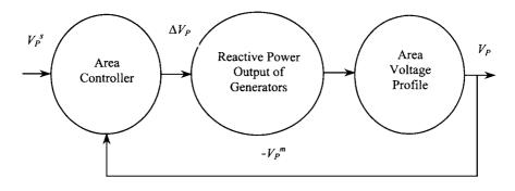
Figure 9.16 Closed-Loop Secondary Voltage/VAR Control
