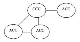
Figure 2.3 Topology of a Four-Processor Parallel Machine
