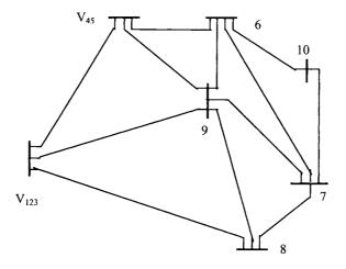
Figure 9.6 System Partitioning Results after Bus 4 and Bus 5 Are Merged
