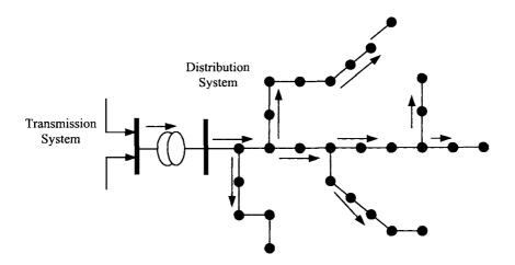
Figure 11.7 Unidirectional Power Flow of Distribution System
