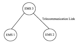
Figure 7.10 Distributed System for State Estimation
