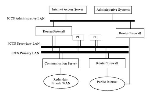
Figure 3.1 Architecture of ICCS LANs
