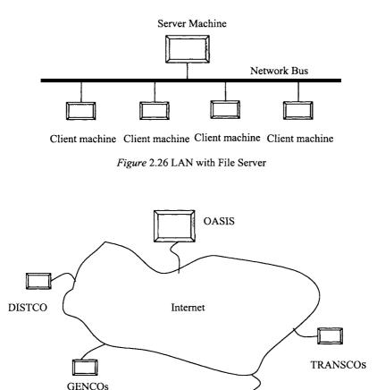
Figure 2.27 Client/Server Architecture of OASIS
