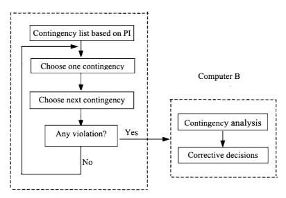
Figure 8.20 Enhanced Online Distributed Security Analysis and Control
