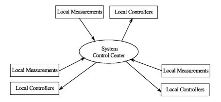
Figure 10.1 Centralized Control Scheme
