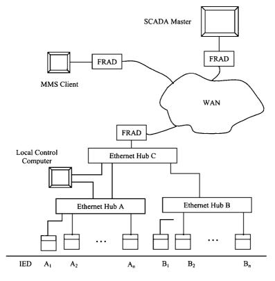
FRAD: Frame Relay Access Device IED: intelligent electronic device
