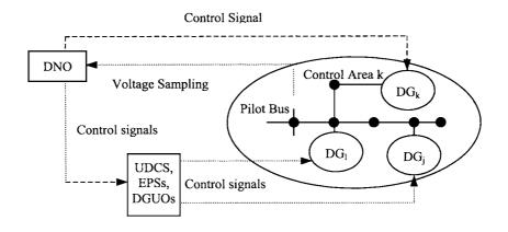
Figure 11.13 Distributed Closed-loop Voltage Control
