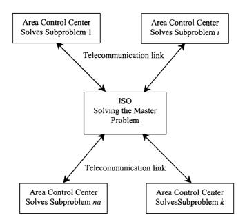
Figure 9.25 Distributed Tertiary Voltage/VAR Optimization Based on WAN
