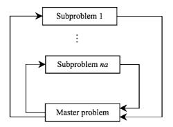
Figure 9.19 Iterative Procedure of the Dantzig-Wolfe Method
