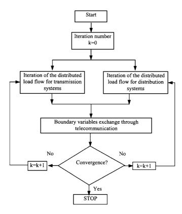
Figure 6.6 Distributed Joint Load Flow Computation
