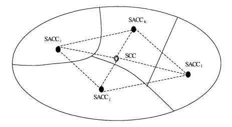
SCC: system control center SACC: subarea control center ---: telecommunication links between control centers
