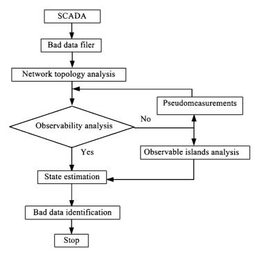
Figure 7.2 Main Components of State Estimation
