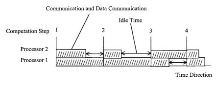
Figure 2.10 Synchronous Computation
