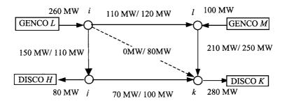
Figure 10.13 Transmission Congestion without Standby Transmission Lines
