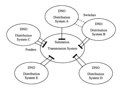
Figure 11.4 Distributed Processing of Distribution System
