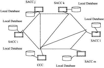
Figure 2.28 Distributed Database of Power Systems
