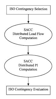
Figure 8.14 Distributed Computation of PI Based on Distributed Load Flow
