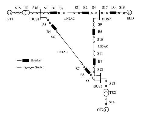
Figure 4.9 Three-Bus Example System
