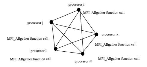
Figure 2.25 MPI\_Allgather Application In Parallel Load Flow Computation
