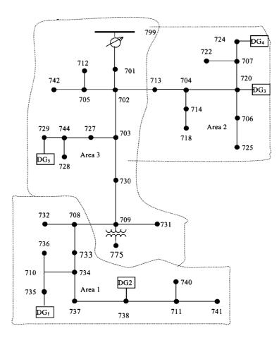
Figure 6.9 Distribution System with Distributed Generation
