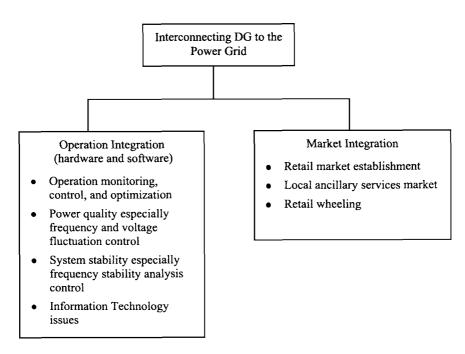
Figure 11.2 Integration of DG into Power Grids
