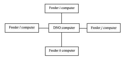
Figure 2.17 Distributed System for Distribution Network
