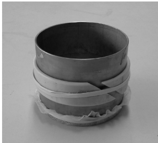
FIGURE 7.1 The lower test cylinder extended to double its height by putting a second test cylinder on top, held in place by using a clamp and a rubber. The test cylinder and rim (second holder) are then filled with a few gentle taps to avoid large voids and create an even filling. The sample is brought to a specific suction force and finally the rim or top cylinder is removed and the excess material is wiped or scraped off with a rigid blade. After weighing, drying and weighing, the bulk density is calculated (see also Plate 19).
