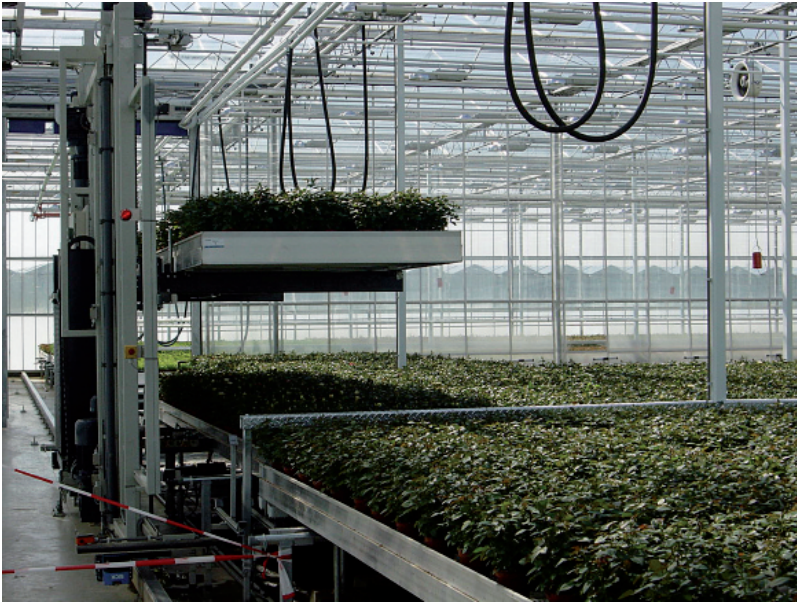
PLATE 15 Movable benches can be transported out of the greenhouse bay to another place. Mostly the pipe-rail system is used; In some applications a robotic lift is used to pull out an entire individual bench for rapid movement to another location (see also Figure 5.22, p. 190).
