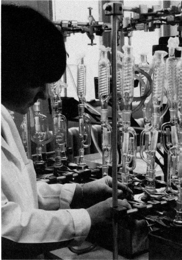
Fig. 2. The Soxhlet extraction of alkaloids from Catharanthus roseus .
