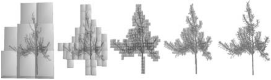
Figure 9.10 Box method applied to a digitized leafy tree in 3-D. The geometry of the plant varies as a function of the scale \delta (size of a grid element).
