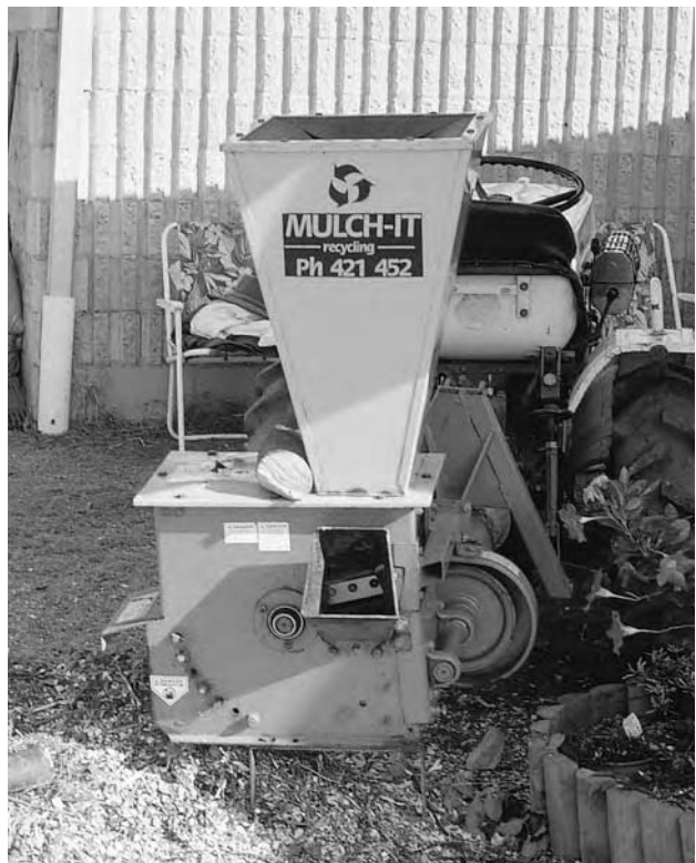
Figure 9.8: Mulchers can be useful for disposing of prunings and other organic material. This small mulcher can be mounted to the back of a tractor.
