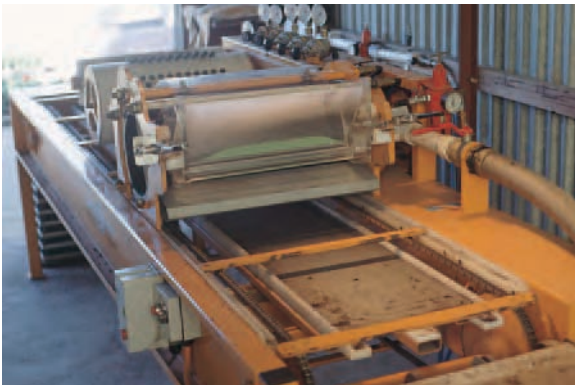
Figure 7: Seeding machine in a large production nursery.
