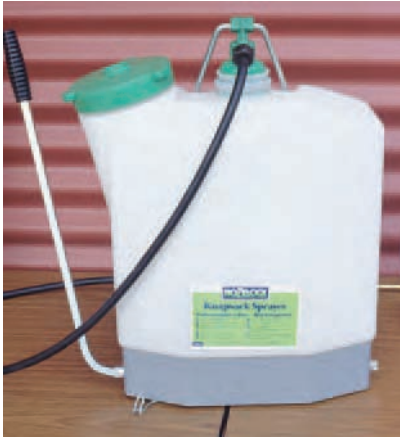
Figure 17: Knapsack-type sprayers like this are convenient in the nursery as they can be carried to almost any location and are simple to use.
