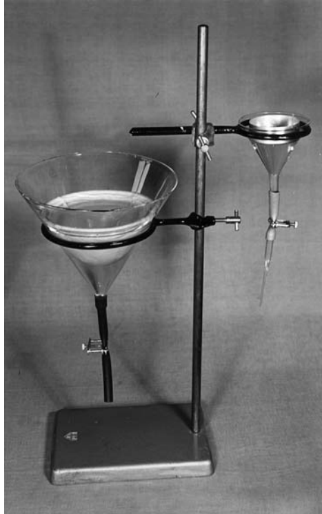
Figure 4.2 Baermann funnels – a simple apparatus for enumerating nematodes; on the left with a cloth bag containing the sample and on the right with a gauze sieve (courtesy of C. C. Doncaster, Rothamsted Research)
