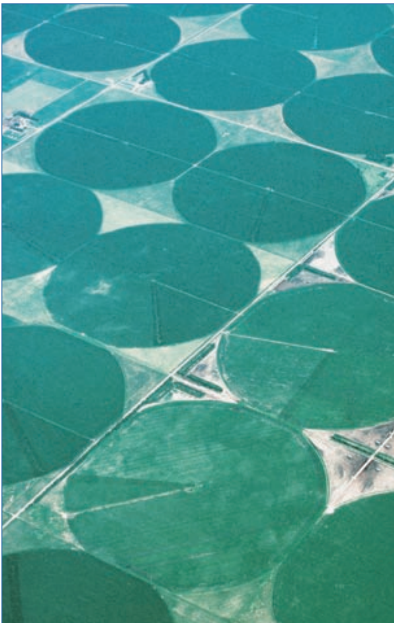
Figure 4.3 Center pivot irrigation creates circular farms such as the ones seen above. Center pivot irrigation is a type of crop irrigation in which equipment rotates around a fixed point. Computer-controlled center pivot irrigation systems allow farmers to operate from a remote location.
