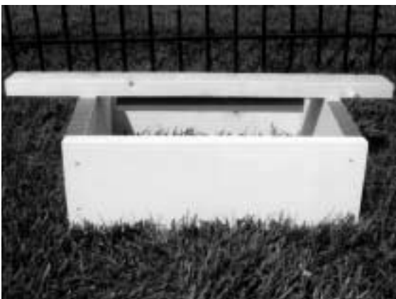
In this picture the die is screwed to the form in the correct position so that a slot will be formed.
