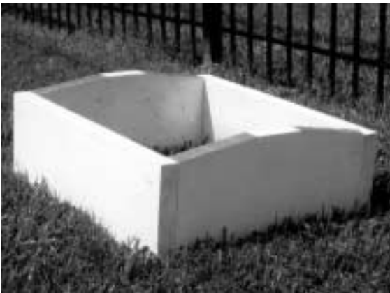
A wooden form constructed of 2x12 lumber makes an excellent material for making replacement bases. The shaded areas are angled away from the center so when the cement dries and the base is placed into service, water will run away from the marker.
