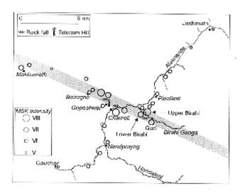
**Figure 5.** Intensity of shaking observed at various locations around Chamoli. Shaded portion shows the trend of the fault as per the fault plane solution which is consistent with the damage distribution.
