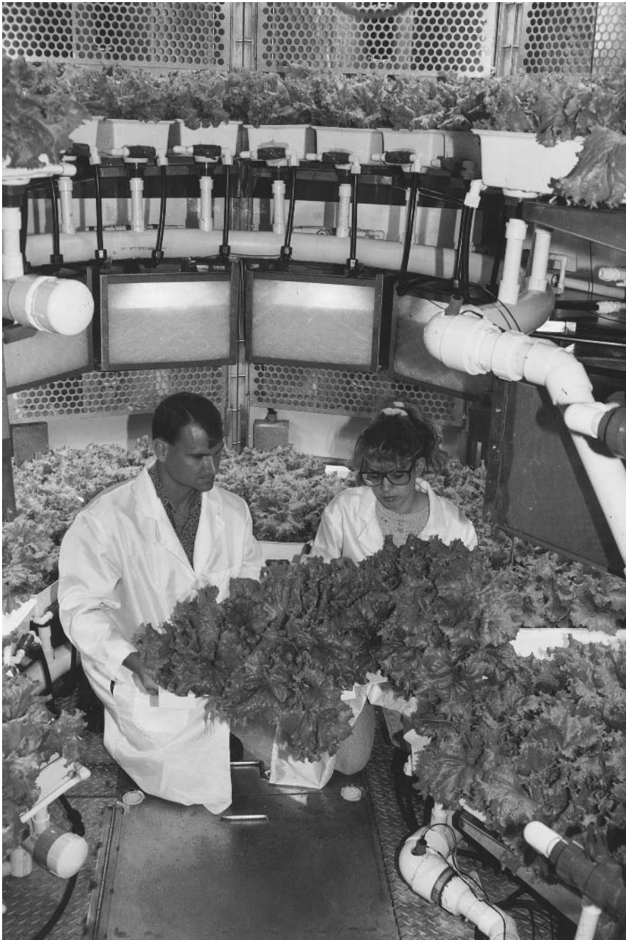
Figure 1 NASA's Biomass Production Chamber located at Kennedy Space Center, Florida. The chamber provides 20 m 2 of growing area in a closed volume of 113 m 3 for testing crop growth and yield for life support applications.
