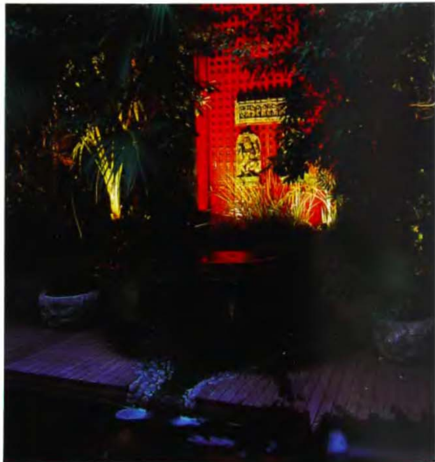
above: Underwater uplighting of the waterfall produces shimmering illumination of the brick structure, while crosslighting of the water staircase adds a sparkling sheen to the trickling of the water running down.
