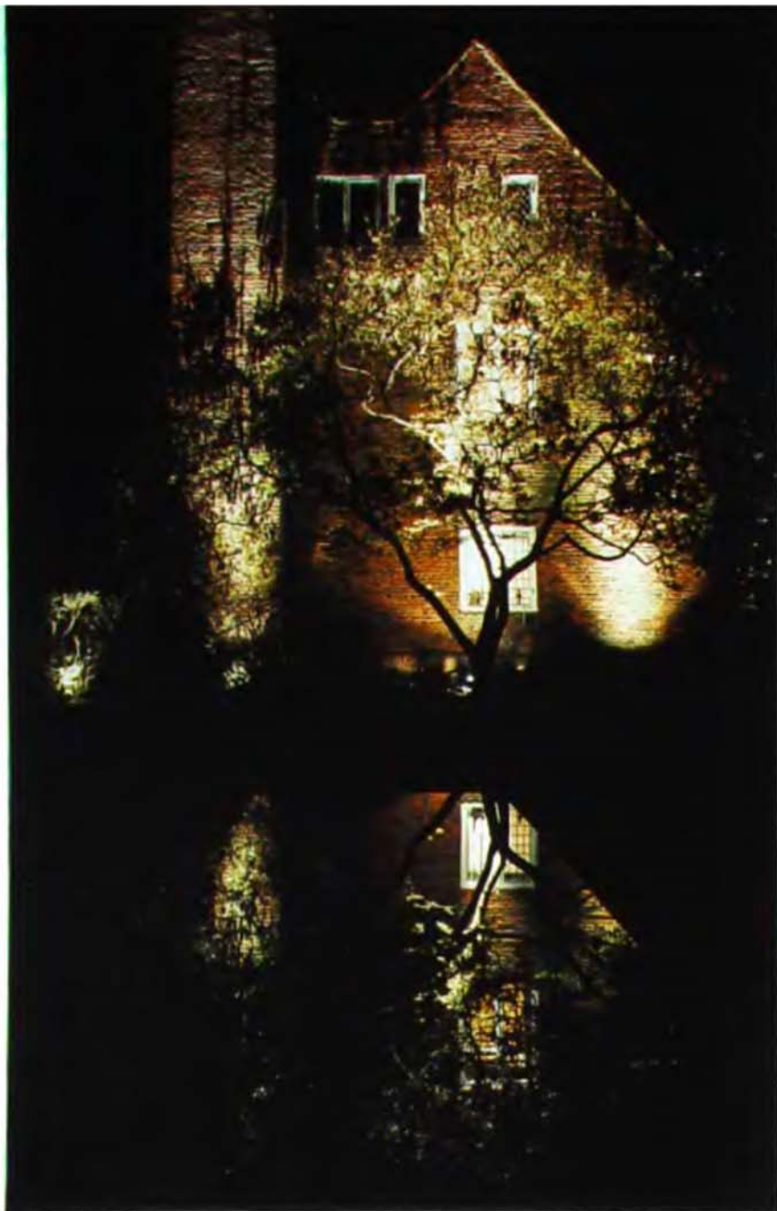
left: Grazing up the house wall emphasizes the texture, as well as the colour of the brickwork, while also silhouetting the magnolia tree. The whole view is reflected in a rectangular pond to be enjoyed from the temple. (see page 61).
