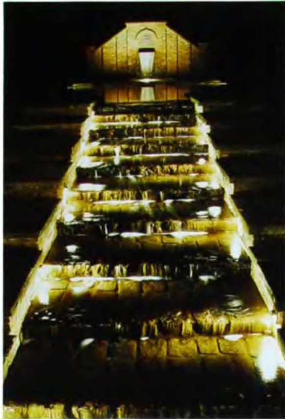
above: Underwater uplighting of the waterfall produces shimmering illumination of the brick structure, while crosslighting of the water staircase adds a sparkling sheen to the trickling of the water running down.
