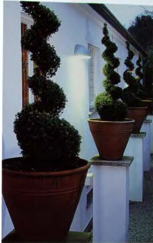
above: White walls have a high reflectance; relatively low levels of light can be used to light the walls and throw the spiral topiary into silhouette.
