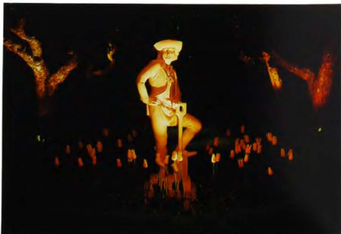
below: The light coloured statue and white tulips are highly reflective with relatively low power lighting. Gentle uplighting and moonlighting of the avenue of apple trees behind adds depth to the view.
