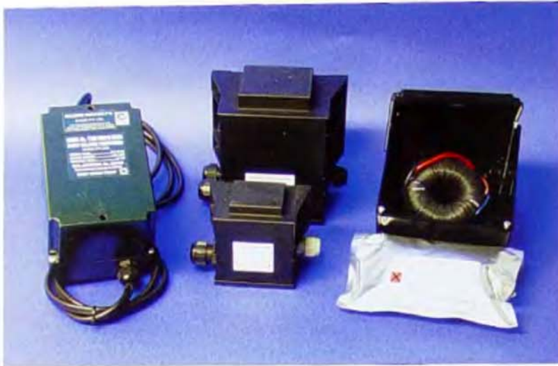
left: Examples of garden lighting transformers: from left – transformer in weatherproof wall-mounting box with cable input and output; transformer sealed into wall-mounting enclosures with cable entries; ground-burial transformer kit with polyurethane potting kit for on-site sealing.
