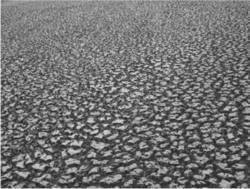
Figure 7.9. A sample of freezing-and-thawing treated sludge from anaerobic digester. (Courtesy of Falke Bruinsma at http://photos.innersource.com )
