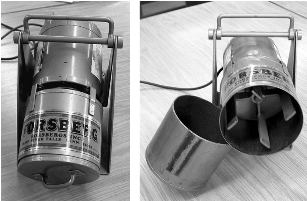
Fig. 17.11. The laboratory scarifier for seed with hard seed coat or thick dried fruit at the Ornamental Plant Germplasm Center.
