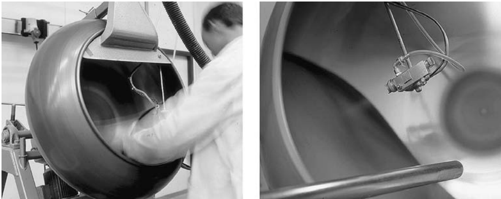
Fig. 13.9. Pelleting of flower seeds in a pelleting pan (left) and a detail of the addition of water during the process (right).
