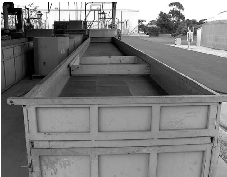
Fig. 11.12. Tunnel dryer commonly used for seed drying.
