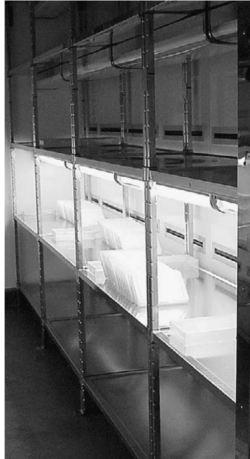
Fig. 14.5. In walk-in germination chambers, lights may be installed on the walls or overhead.
