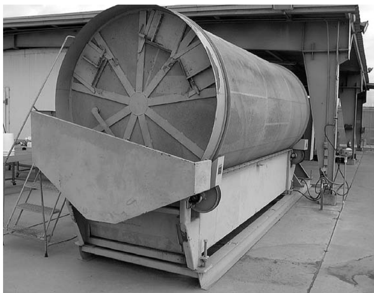
Fig. 11.13. Rotary dryer used for drying plant materials.
