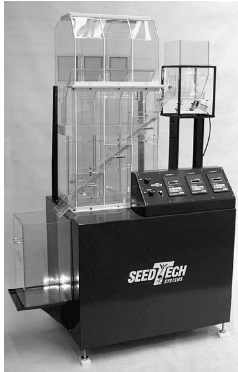
Fig. 12.10. A multi-cut air column with individual air control for each column. Four density fractions can be obtained in each run.
