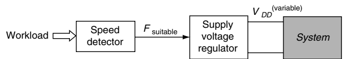
FIGURE 5.16 Variable Voltage Scheme. A speed detector is used to sense the suitable frequency and execute some workload; consequently, the supply voltage regulator will generate a suitable supply voltage level for this specific frequency.
