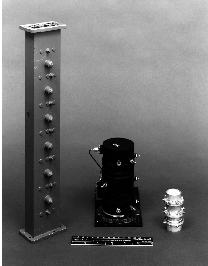
FIGURE 6.33 Size comparisons between traditional cavity filters and dielectric resonator filter (single mode rectangular waveguide filter, dual mode circular cavity filter, and dual mode dielectric resonator filter are shown).
