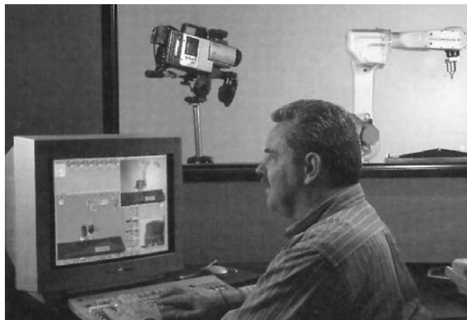
A video camera provides a Deneb Robotics engineer with a view of the robot. (Photo courtesy of National Aeronautics and Space Administration.)
