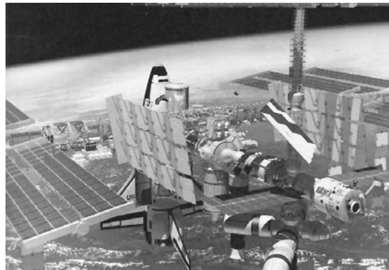
This concept view is of the station from the opposite (aft port) end. In the foreground (lower right) is the Russian service module, with living and working room for three crew members. Next, toward the center of the photo, is the FGB energy block, then (near the orbiter) the U.S. laboratory module. The vertically mounted cylinder below it is the U.S. habitation module. (Photo courtesy of National Aeronautics and Space Administration.)
