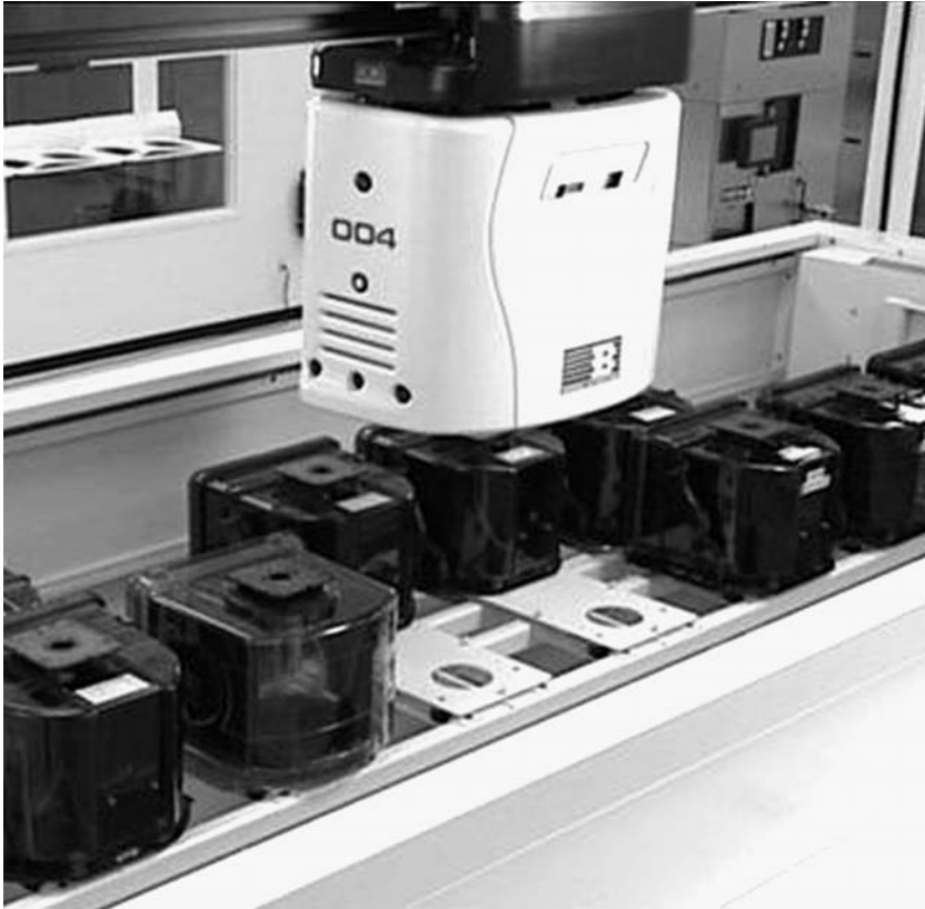
FIGURE 33.19 Example overhead hoist transport (OHT) vehicle (OHV). (Photograph courtesy of Brooks Automation.)
