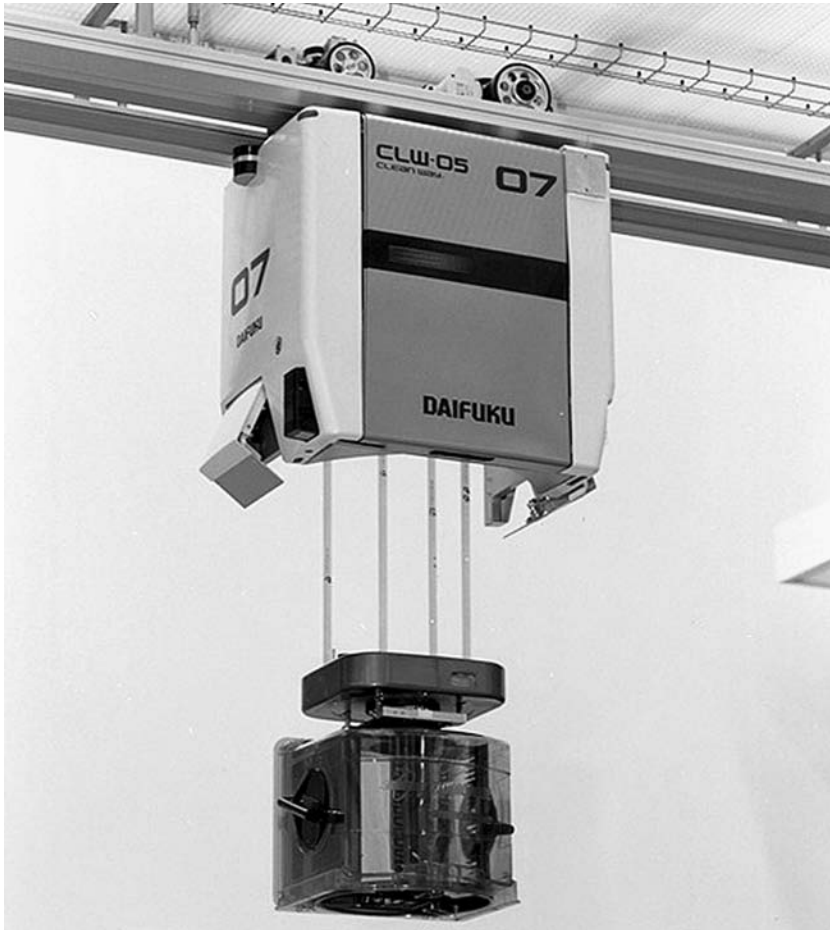
FIGURE 33.20 Example overhead hoist transport (OHT) vehicle. (Photograph courtesy of Daifuku Co., Ltd.)
