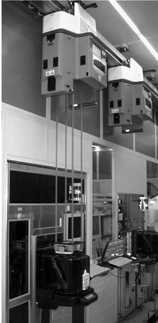
FIGURE 33.25 Overhead hoist vehicle (OHV) on monorail track installed in the ceiling and picking up a FOUP from a tool load port. (Photograph courtesy of Intel Corporation.)
