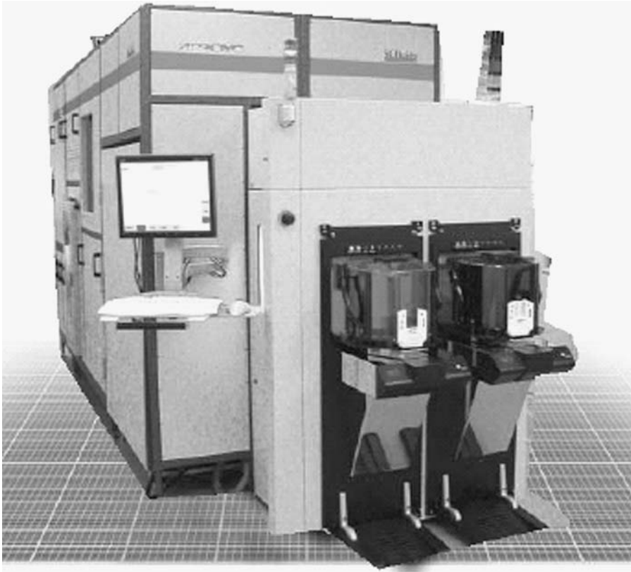
FIGURE 6.13 The 300-mm Arroyo system for cleaning semiconductor chips. (From Rothman, L., Annual Retreat , 2003. Available online http://www.gscn.net/event/images/Speech-6.PDF .)
