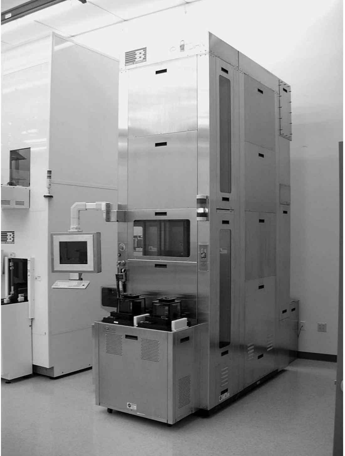
FIGURE 33.17 Example bare reticle stocker. (Photograph courtesy of Brooks Automation, Inc.)
