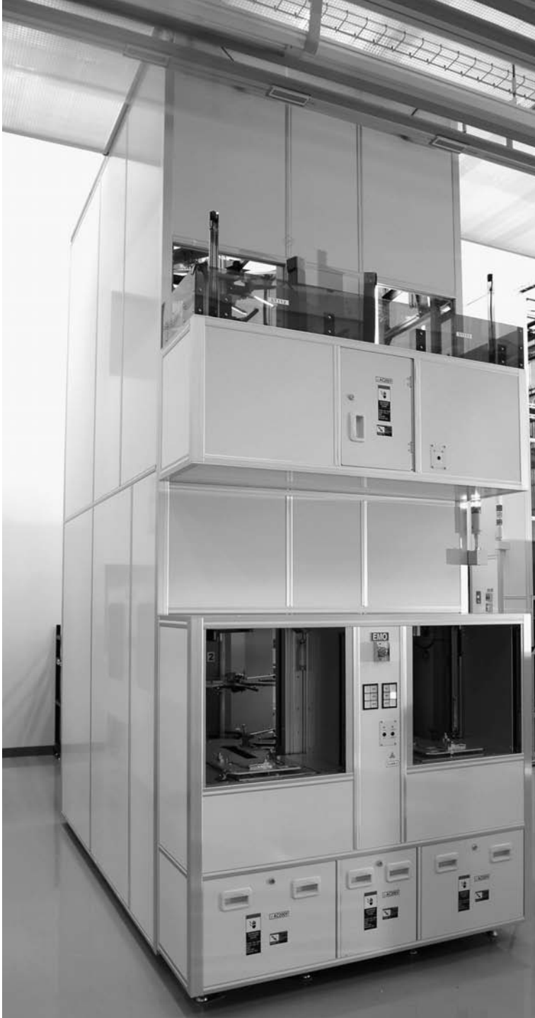
FIGURE 33.14 Example inter-level lifter-silo stocker. (Photograph courtesy of Daifuku Co., Ltd.)
