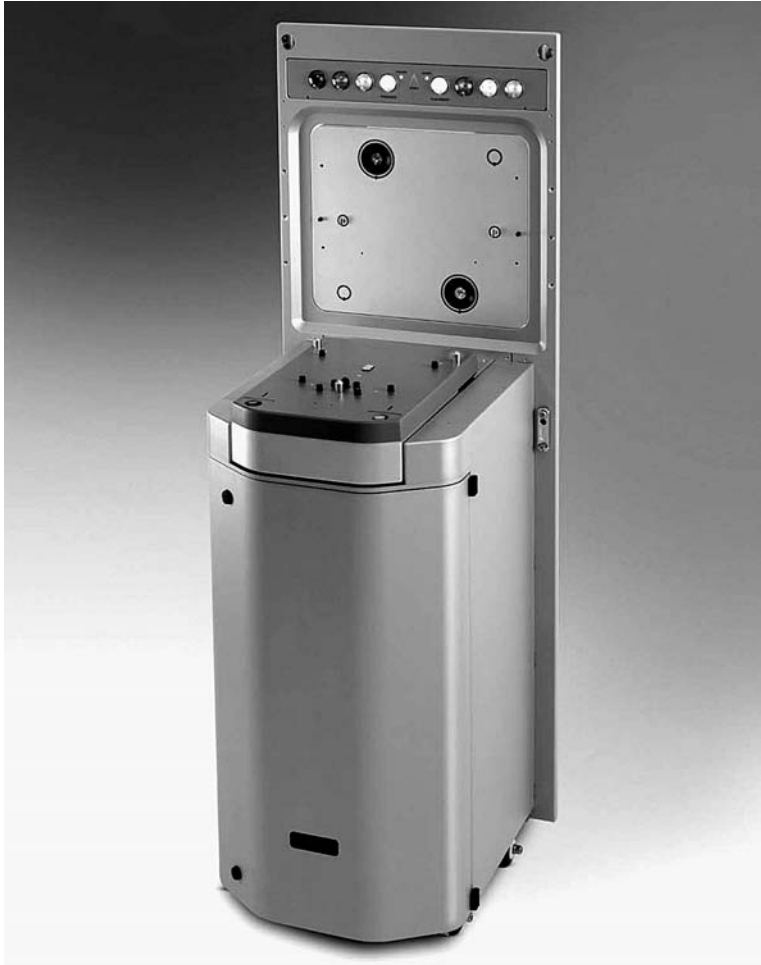
FIGURE 33.22 Example 300 mm process tool load port with front opening interface mechanical standard (FIMS) port and status indicator lights shown. (Photograph courtesy of Asyst Technologies, Inc.)
