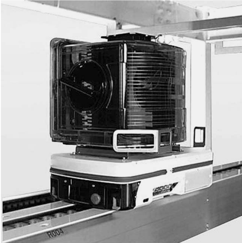
FIGURE 33.13 Example interbay overhead shuttle (OHS) vehicle. (Photograph courtesy of Asyst Shinko, Inc.)
