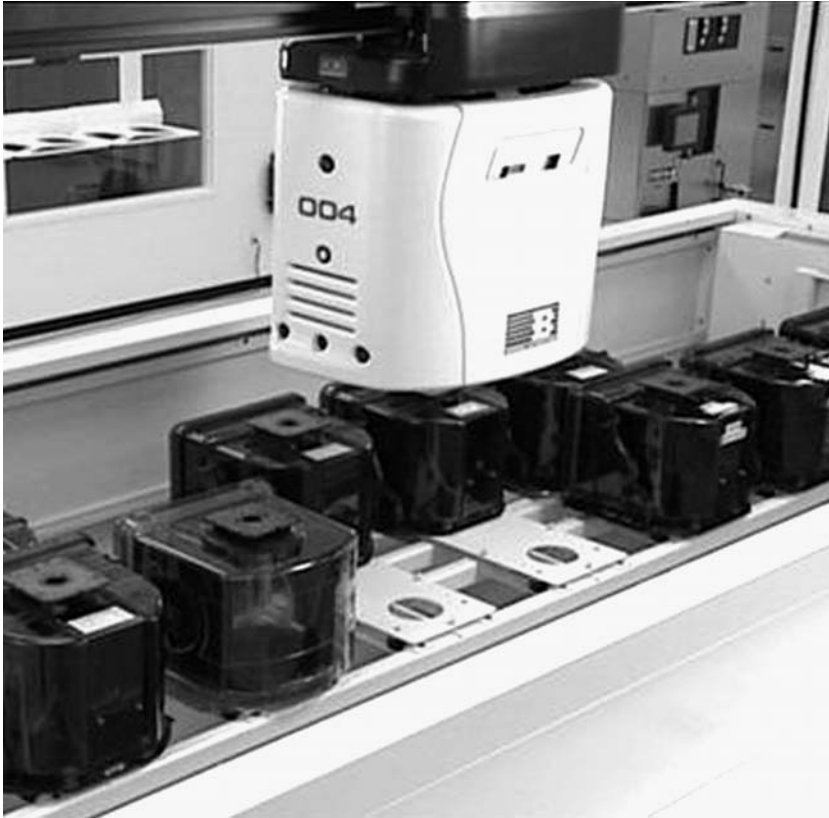
FIGURE 33.16 FOUF carousel stocker top view. (Photograph courtesy of Brooks Automation, Inc.)
