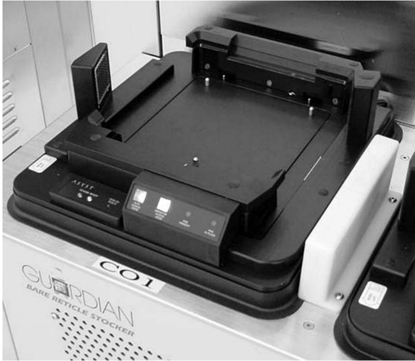
FIGURE 33.23 Example RSP load port with pod lead-in fixtures and radio frequency identification (RF ID) tag reader unit at right side. (Photograph courtesy of Brooks Automation, Inc.)
