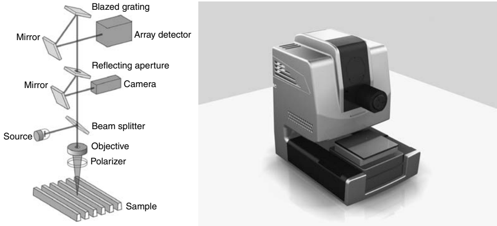
FIGURE 20.51 Normal incidence ellipsometry (NANOmetrics, Inc.). (From Hoobler, R. J., In Handbook of Photomask Manufacturing Technology , Taylor & Francis Group, 433–55. Boca Raton, FL, 2005.)
