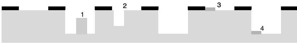
FIGURE 20.62 Phase related defects on Alt.PSM. (From Rosenbusch, A., and S. Hemar, In Handbook of Photomask Manufacturing Technology , Taylor & Francis Group, 589–98. Boca Raton, FL, 2005.)
