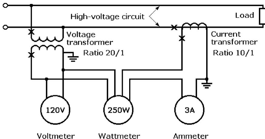
**Figure 3-19** Instrument transformer connections: voltmeter, wattmeter, and ammeter.
