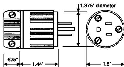
2-pole, 3-wire grounding dead plug, 15 A, 125 V
