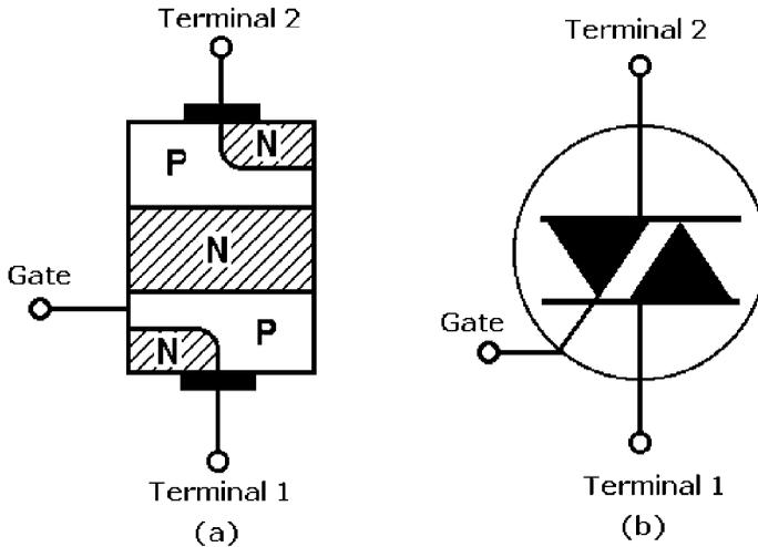
**Figure 3-30** Triac: (a) functional diagram; (b) schematic symbol.
