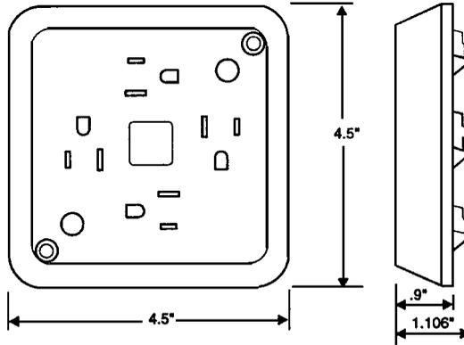
2-pole, 3-wire grounding quad receptacle, 15 A, 120 V
