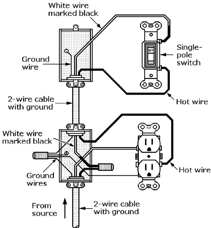
**Figure 7-13** Both outlets of a duplex receptacle are controlled by a single-pole switch. Outlets are “hot” only when the switch is on.
