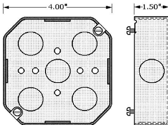
**Figure 6-11** Octagonal metal box with a volume of 15.8 in.<sup>3</sup> can contain wiring for a ceiling luminaire and a yoke or strap with a stud to support it.
