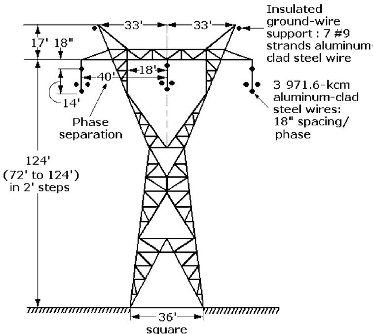
**Figure 2-6** A 500-kV steel self-supporting transmission tower.
