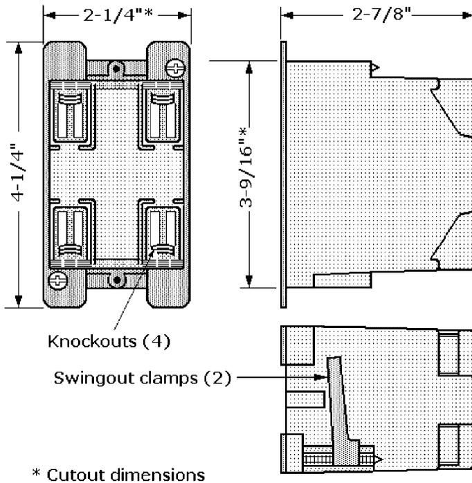
**Figure 6-9** Plastic 4-in.  $\times$  3-in. switchbox for positioning in a wallboard cutout is fastened with swingout clamps. It has a volume of 5.5 in.<sup>3</sup>.
