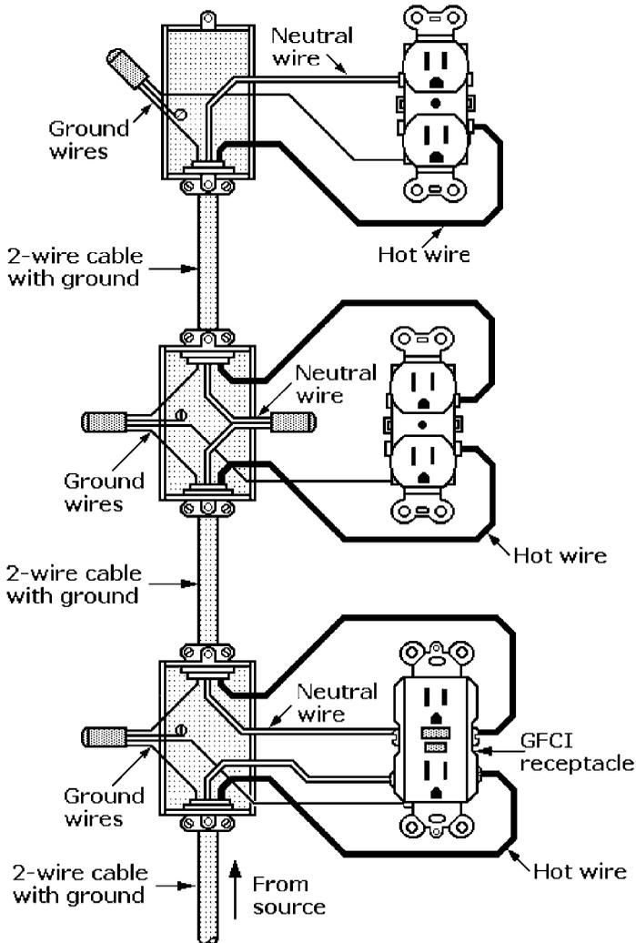
**Figure 7-15** Duplex GFCI receptacle protects two downstream receptacles.
