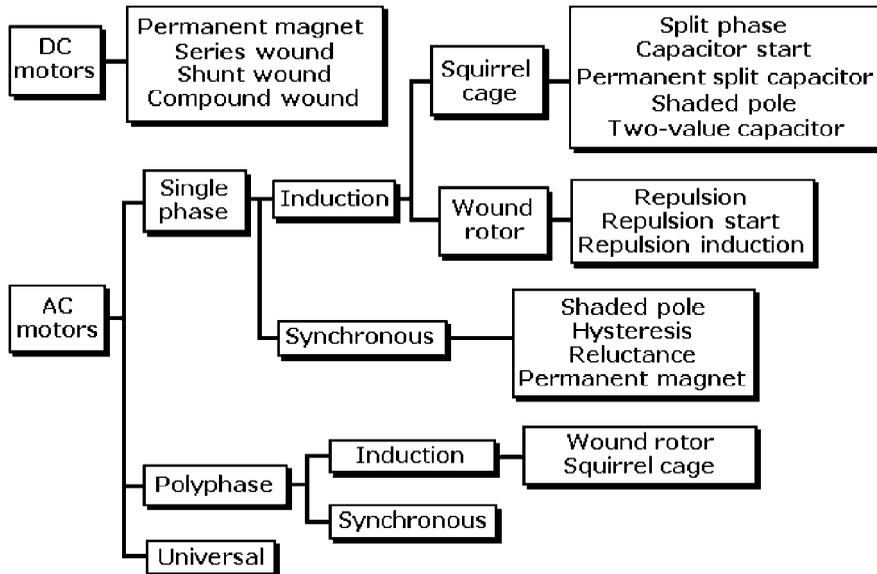
**Figure 10-1** Classification of AC and DC motors.
