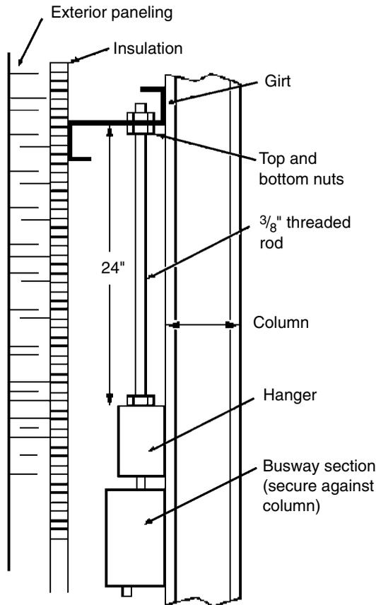
**Figure 1-10** Electrical construction detail for hanging a busway.
