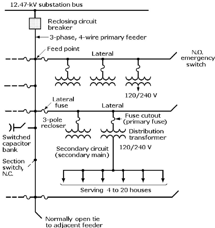
**Figure 4-3** Simplified diagram of a power distribution feeder.
