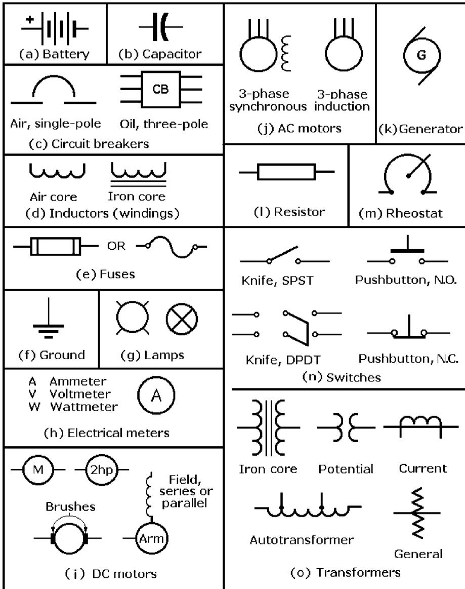
Figure 1-3 Graphic symbols for electrical schematics, Part 1.
