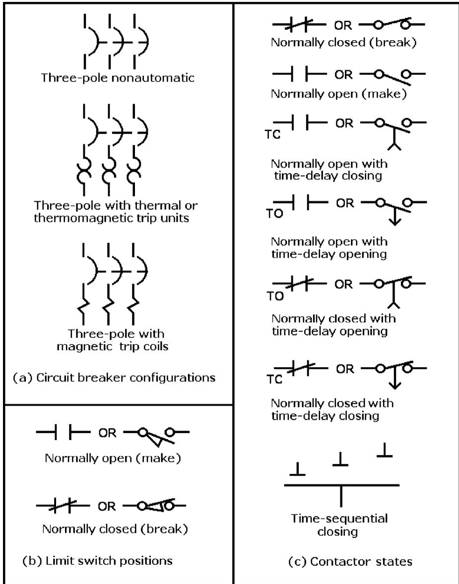
**Figure 1-4** Graphic symbols for electrical schematics, Part 2.
