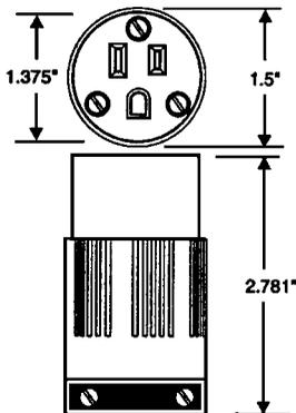
2-pole, 3-wire grounding connectors, 15 A, 125 V
