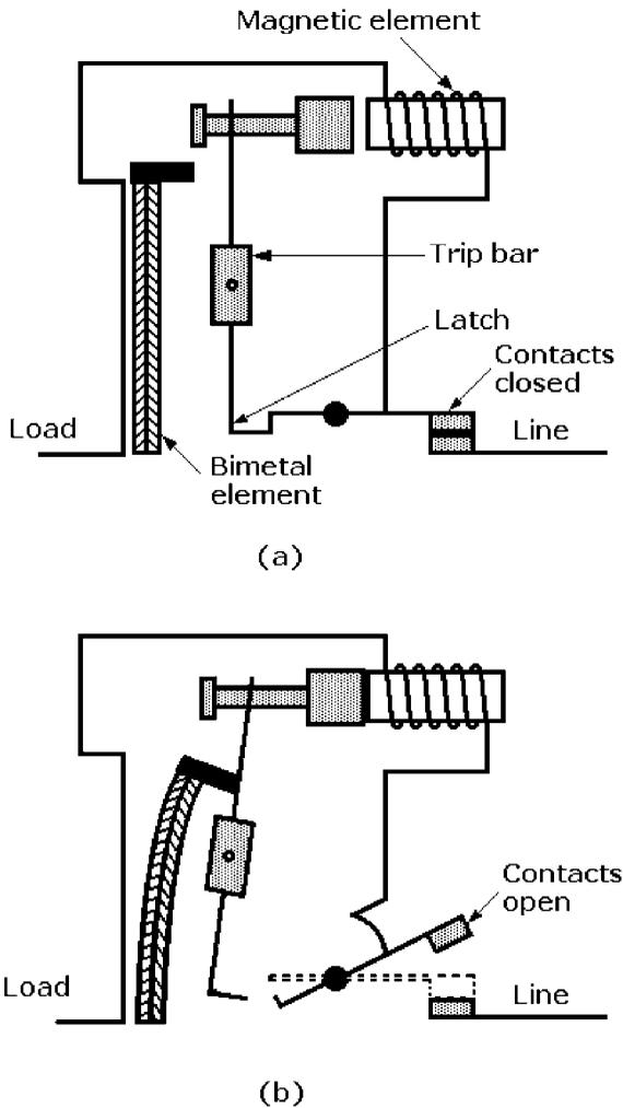
**Figure 5-17** Thermal-magnetic circuit breaker trip latch operation: (a) normal; (b) overcurrent condition.
