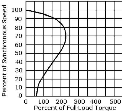
**Figure 10-7** Speed-torque curve for a typical permanent split-capacitor motor.
