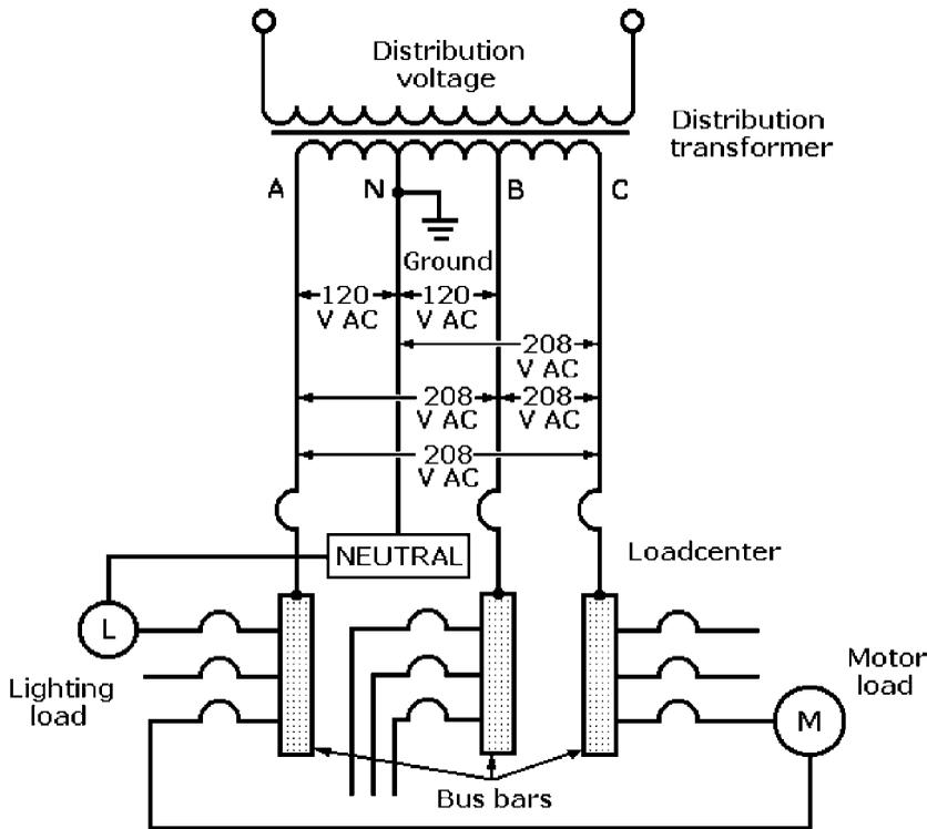
**Figure 5-12** Schematic diagram for a three-phase, four-wire loadcenter.
