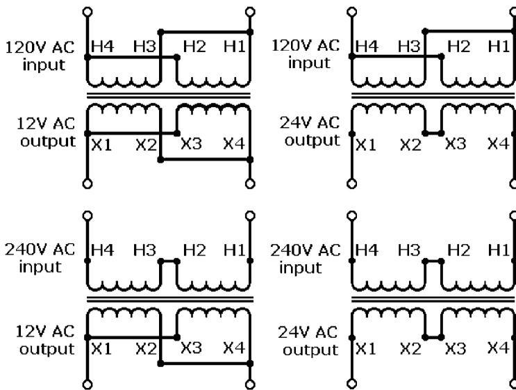
**Figure 3-17** Wiring diagrams for low-voltage, single-phase, buck-boost transformers.
