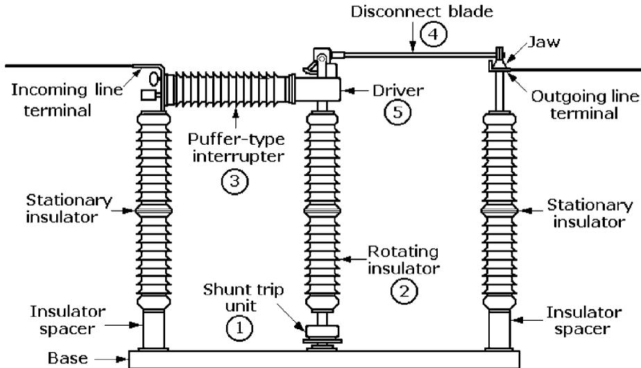
**Figure 3-20** Single pole of a blade-type circuit switcher.
