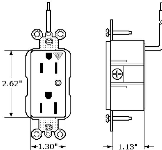
**Figure 12-4** Isolated grounding surge protective duplex receptacle identified by its orange body or an orange triangle on its face.
