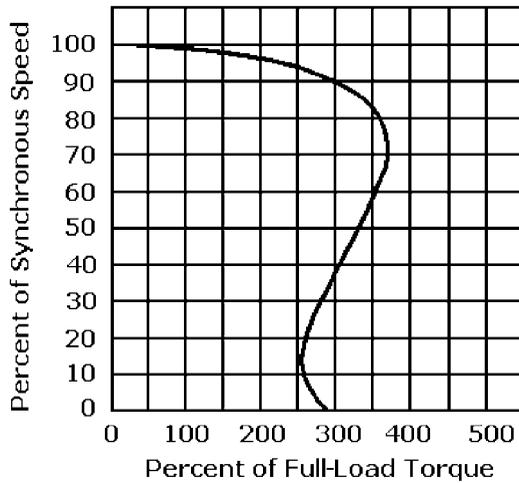
**Figure 10-10** Speed–torque curve for a typical polyphase AC motor.
