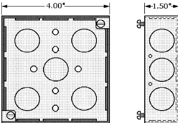
**Figure 6-10** Metal 4-in.  $\times$  4-in. device box with a volume of 22.5 in.<sup>3</sup> can contain two switches or duplex receptacles.
