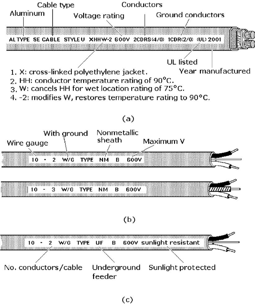
**Figure 6-3** Codes printed on the jackets of cables identify them as: (a) service entrance (SE), (b) nonmetallic (NM), and (c) underground feeder (UF).
