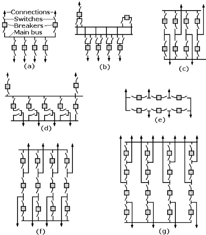
**Figure 4-2** One-line diagrams of substation switching arrangements: (a) single bus; (b) double bus, single breaker; (c) double bus, double breaker; (d) main and transfer bus; (e) ring bus; (f) breaker-and-a-half; (g) breaker-and-a-third.
