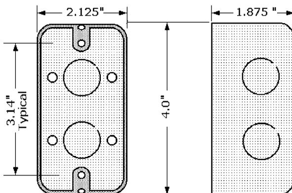
**Figure 6-8** Metal utility 3-in. × 2-in. device box has a volume of 13.0 in.<sup>3</sup>.
