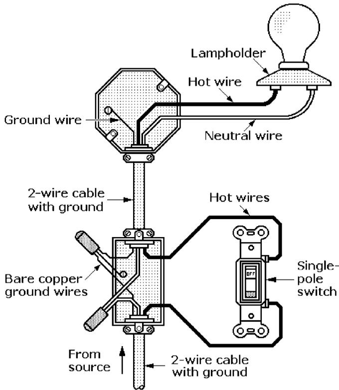
**Figure 7-5** Switch in the middle of the circuit.
