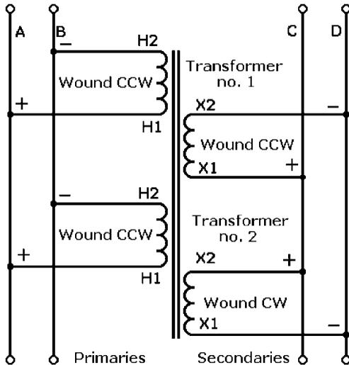
**Figure 3-15** Two transformers connected for parallel operation.
