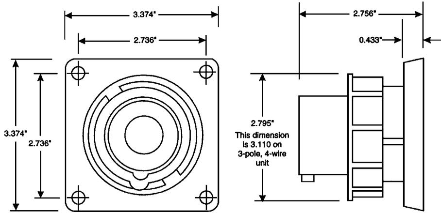
Pin-and-sleeve watertight 20-A, 2-pole, 3-wire and 3-pole, 4-wire inlets have many outline dimensions in common
