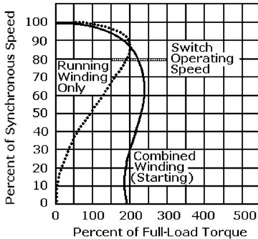
**Figure 10-4** Speed–torque curves for a typical split-phase motor.
