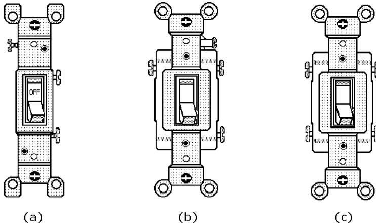
**Figure 7-1** Wall switches can be identified by the number and color of their screw terminals: (a) A single-pole switch has three screw terminals (one grounding); (b) a three-way switch has three screw terminals; and (c) a four-way switch has four screw terminals.
