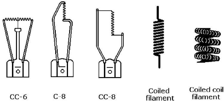
**Figure 8-4** Examples of incandescent lamp filament forms.
