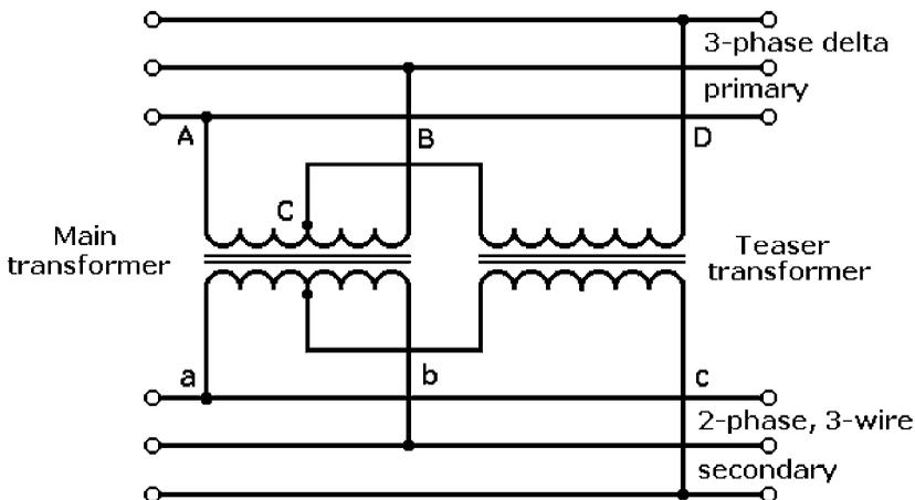
**Figure 3-11** T-connected transformers.
