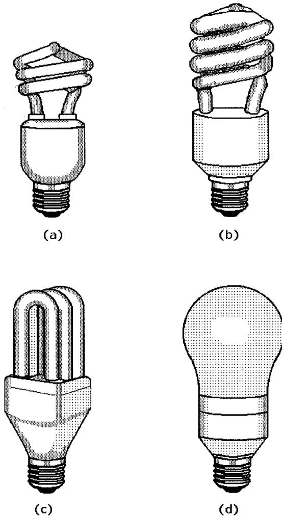
**Figure 8-7** Compact fluorescent lamps (CFLs):
