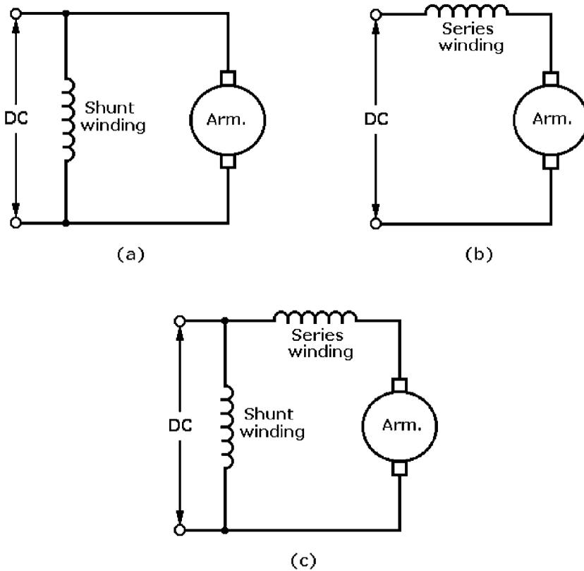
**Figure 10-15** Schematics for three common DC motors: (a) shunt; (b) series; (c) compound.
