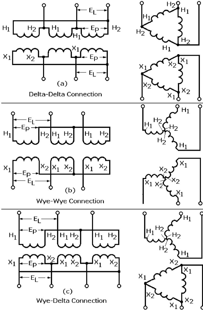
**Figure 3-9** Three-phase transformer connections.
