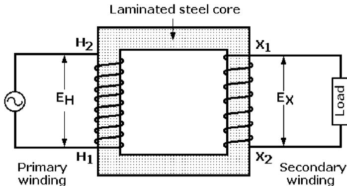
**Figure 3-2** Schematic diagram of a basic transformer.
