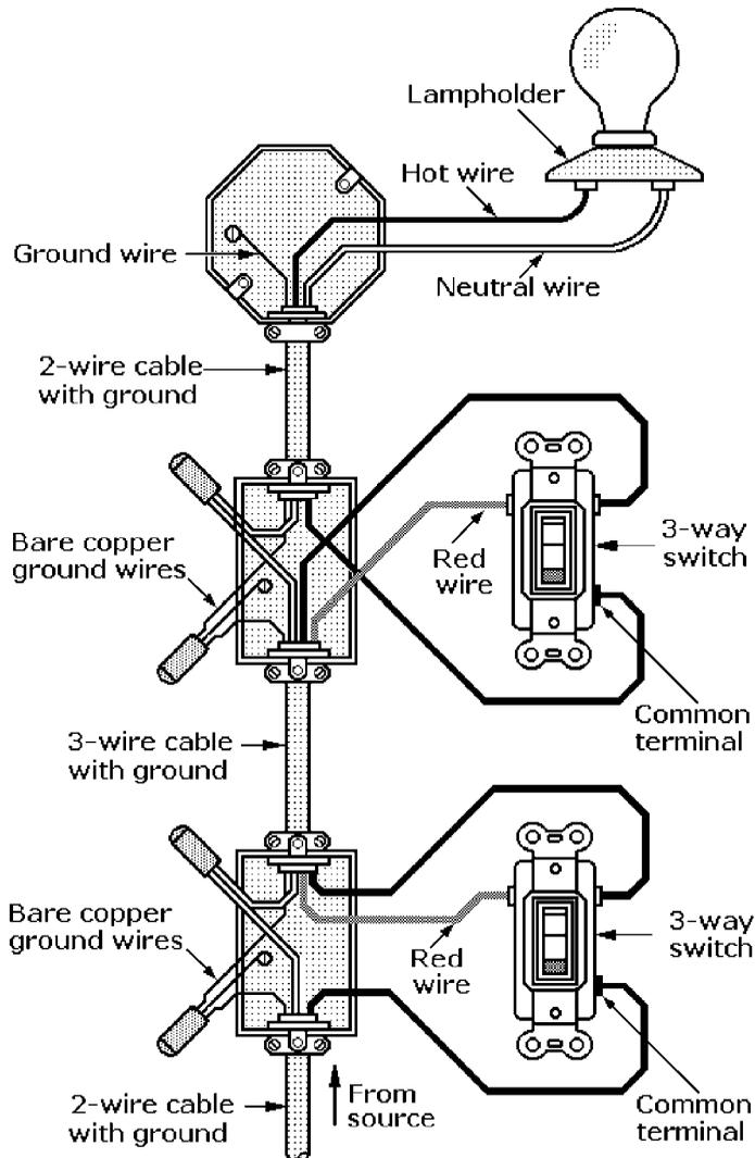
**Figure 7-9** Power goes through a pair of three-way switches to a lampholder at the end of the circuit.
