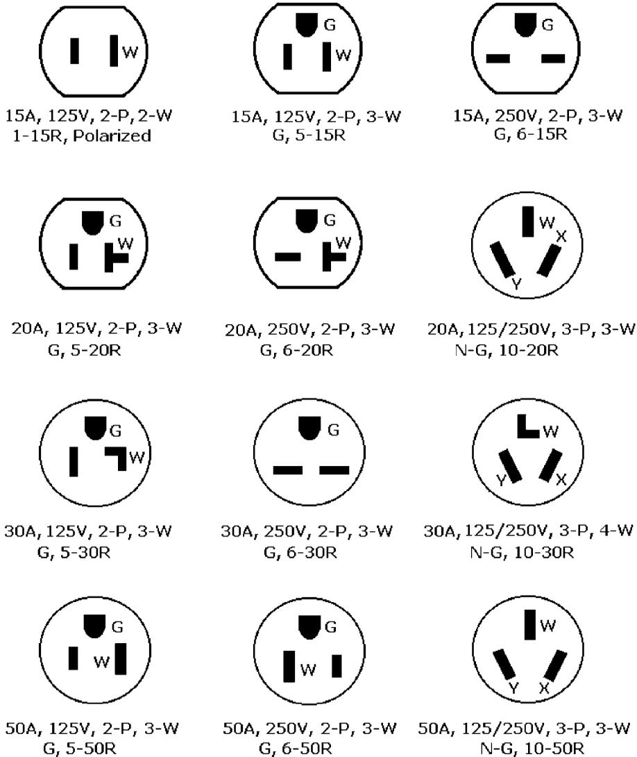
**Figure 6-16** NEMA straight-blade receptacles rated 15 to 50 A and 125 to 250 V AC. Abbreviations: P = poles, W = grounding, N-G = nongrounding. Plug patterns are typically mirror images of receptable patterns.
