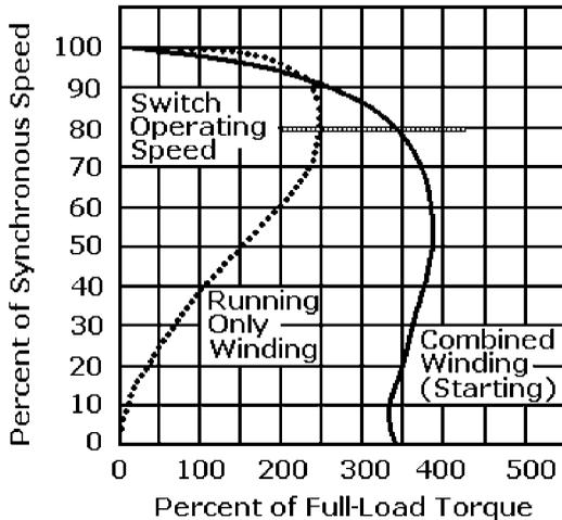
**Figure 10-5** Speed–torque curves for a typical capacitor-start motor.
