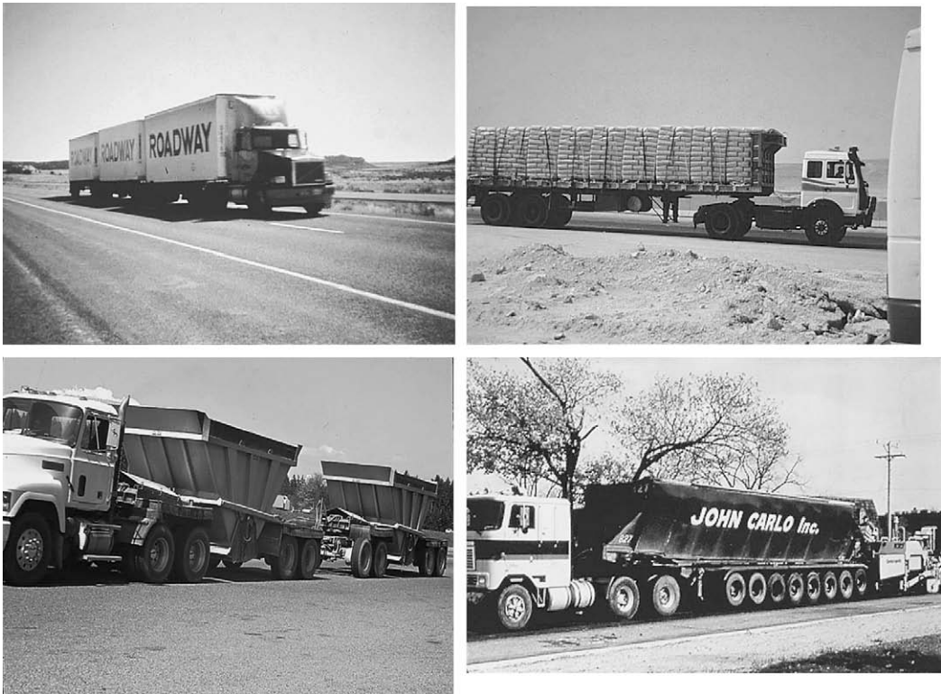
FIGURE 8.3 Trucks with different axle and wheel configurations.
