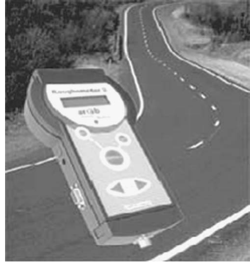
FIGURE 19.63 ARRB roughometer (Source: ARRB, 2005) (Copyright ARRB Group Ltd., 2005).
