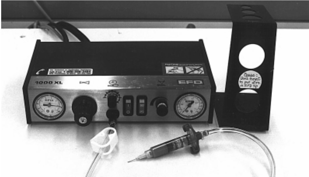
FIGURE 10.12 A semiautomatic dispenser for adhesive application
