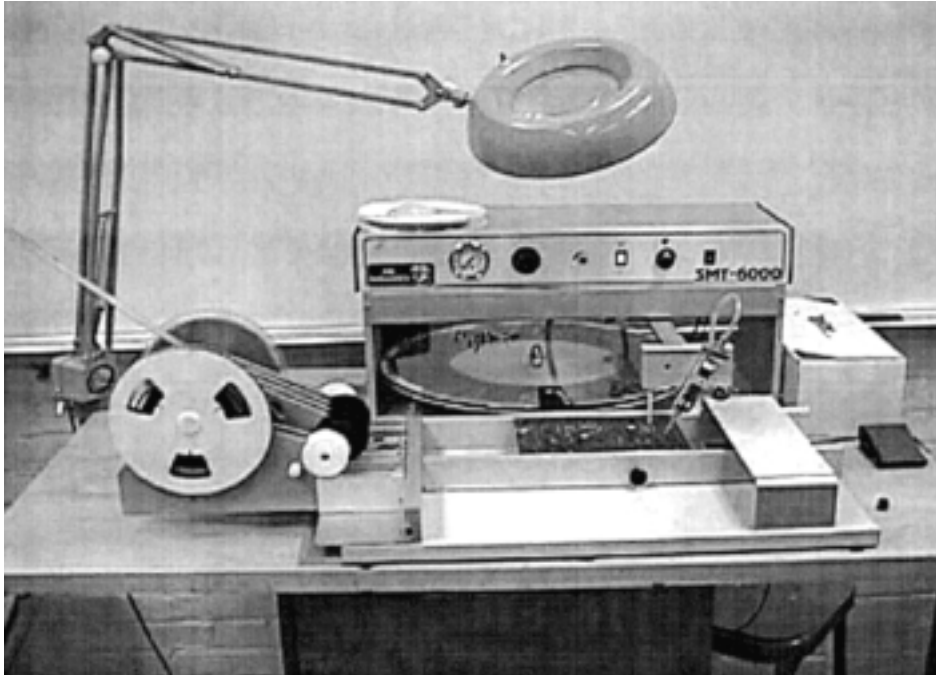
FIGURE 2.25 x-y table for SMT paste and part placement.
