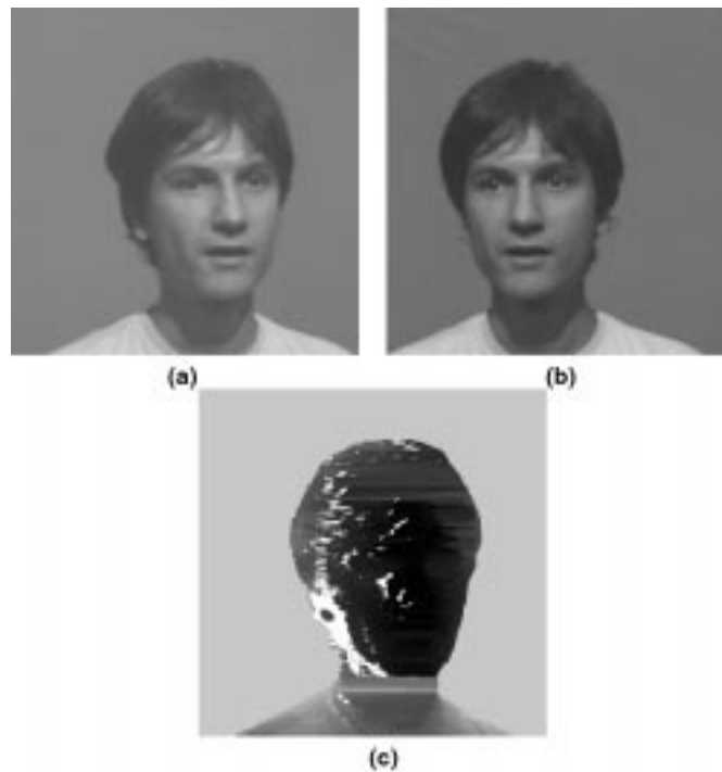
FIGURE 57.4: The left (a) and right (b) view image from a stereoscopic image pair. (c) Disparity field in the stereoscopic image pair represented as gray values (black is foreground, gray is background, white is occlusion).
