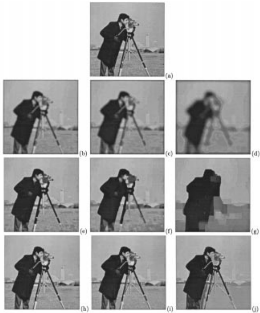
FIGURE 74.5: (a) Original image and its multiscale smoothings via: (b,c,d) Gaussian convolution at scales 2, 4, 16; (e,f,g) close-opening by a square at scales 2, 4, 16; (h,i,j) close-opening by reconstruction at scales 2, 4, 16.
