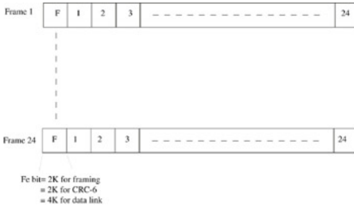
Figure 26-6: Extended Superframe Format improves uptime and error checking
