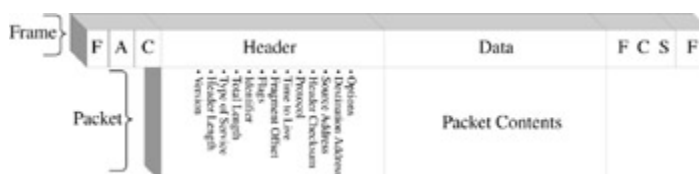
Figure 29-5: The relationship between the frame and packet
