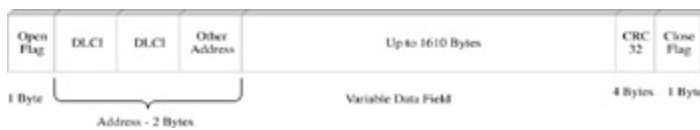
Figure 10-4: A Frame Relay frame
