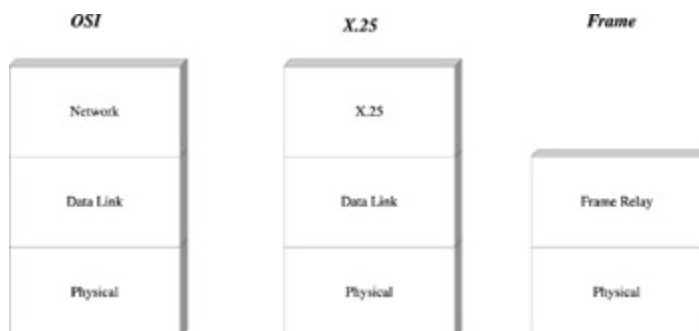
Figure 10-7: OSI compared to Frame and X.25 stacks
