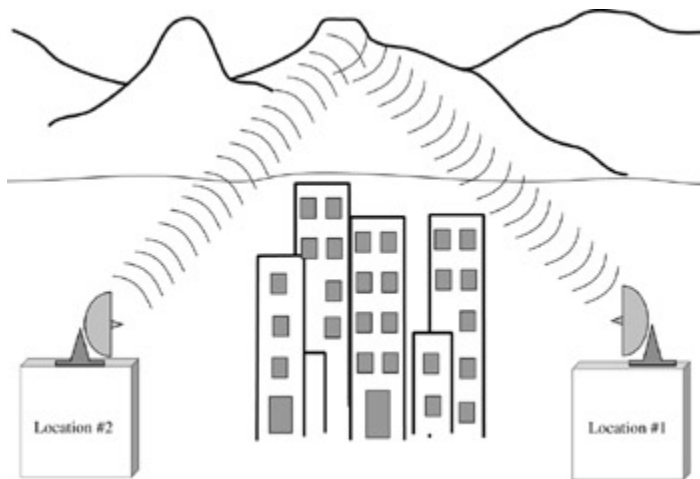
Figure 17-6: Obstacle gain uses a bounced signal off a natural obstacle, such as a mountain.
