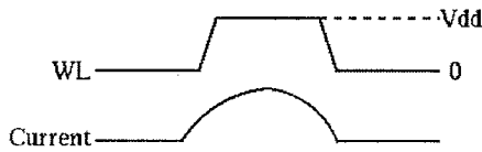
FIGURE 49.3 Word-line signal and current reduction by pulsing the word line
