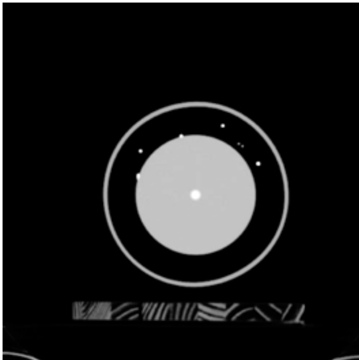
FIGURE 16.22 Conventional CT image of a stationary phantom. (Reprinted by permission of IEEE © 2000.)
