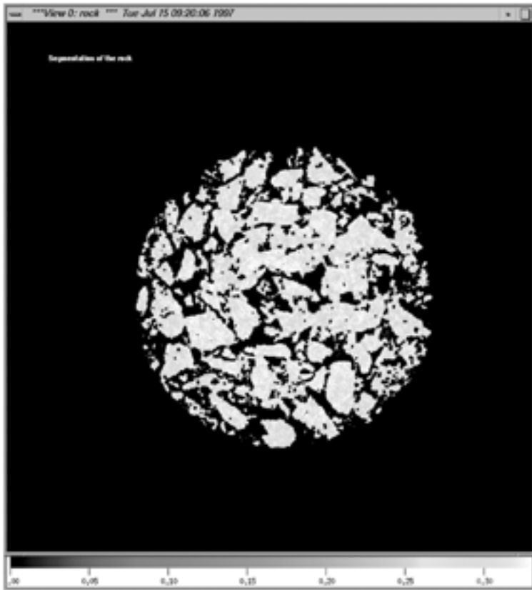
FIGURE 15.17 Segmentation results of the rock within the asphalt sample for the slice plane shown in Figure 15.16 .
