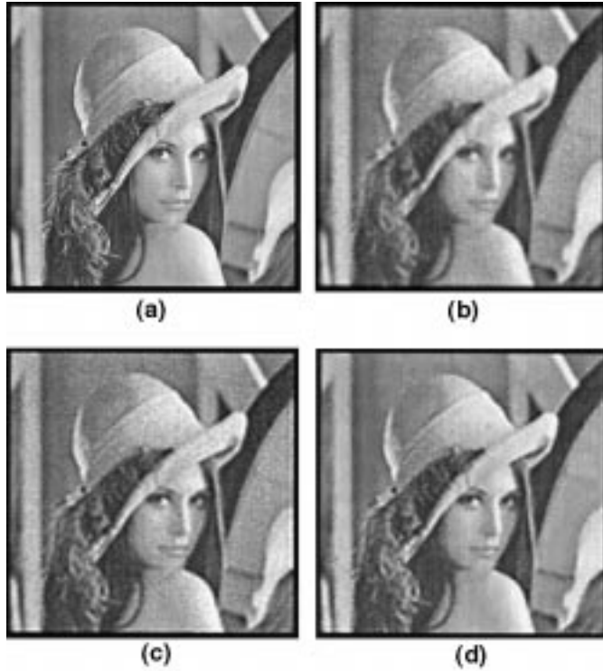
FIGURE 25.4: (a) Original image. (b) Degraded image at 25 dB SNR. (c) Restored image using Kaczmarz iterations. (d) Restored image using the modified Kaczmarz algorithm in a POCS framework. (Courtesy of IEEE: Kuo, S.S. and Mammone, R.J., Image restoration by convex projections using adaptive constraints and the l_1 norm, IEEE Trans. Signal Process. , 40, 159–168, 1992.)
