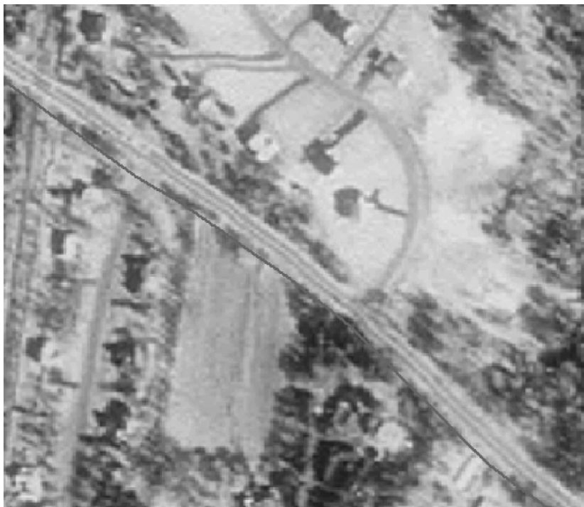
Figure 6.3 Poor vector fit with DOQQ.
