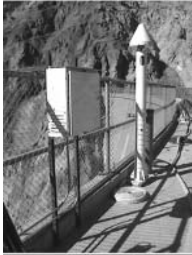
Figure 10.5 GPS for monitoring bridge deformation. (Courtesy of Magellan Corporation.)
