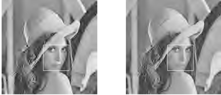
FIGURE 18.3 The trade-off between image quality (at a compression ratio of 80:1) and robustness. (a) Positively modulated image after compression; (b) negatively modulated image after compression. ( Photo: Copyright © 1972 by Playboy magazine. With permission.)
