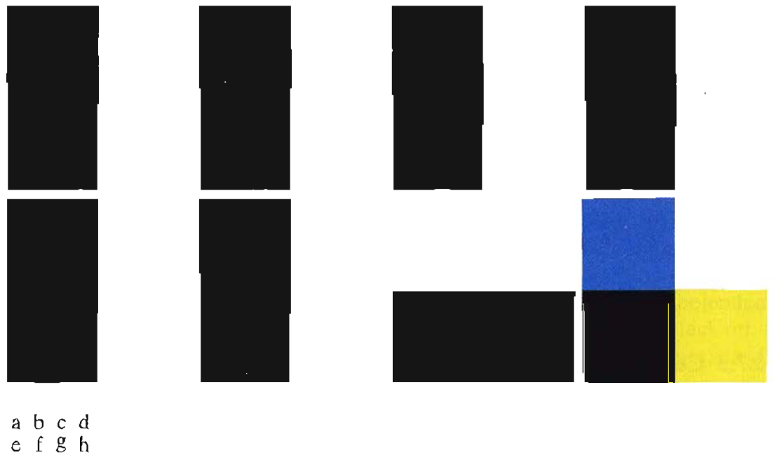
FIGURE 6.45 (a)–(c) R , G , and B component images and (d) resulting RGB color image. (e)–(g) R , G , and B component images and (h) resulting RGB color image.
