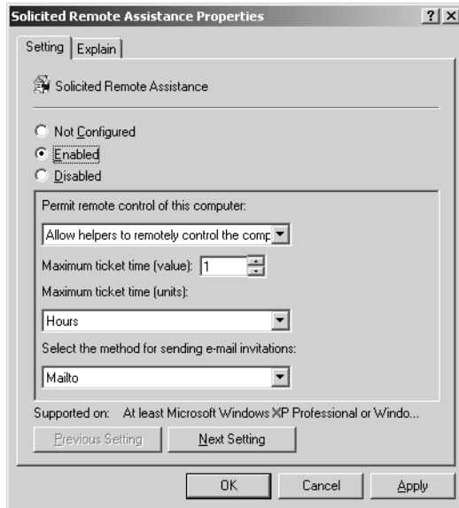
Figure 13-10 The Solicited Remote Assistance Properties dialog box
