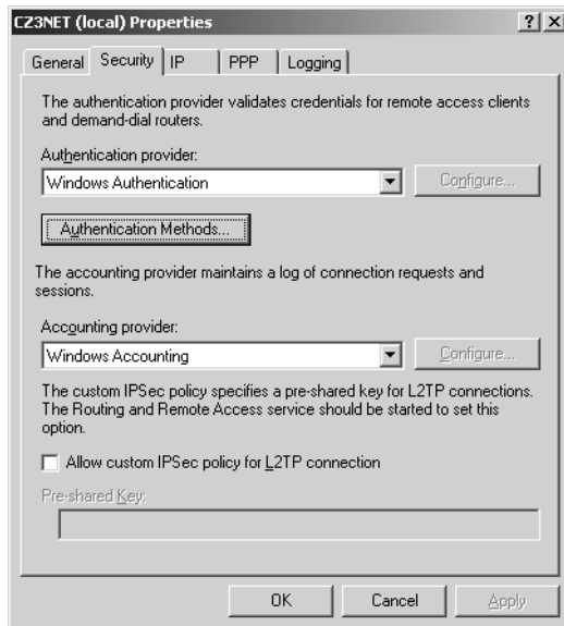
Figure 5-7 The Security tab in a Routing and Remote Access server's Properties dialog box
