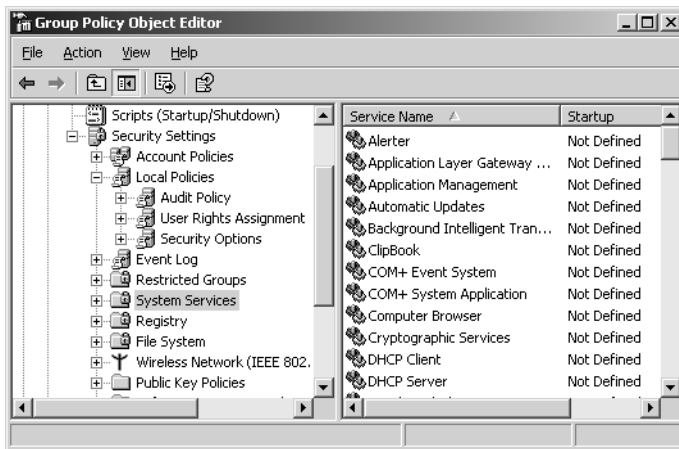
Figure 9-7 The System Services container in the Group Policy Object Editor console
