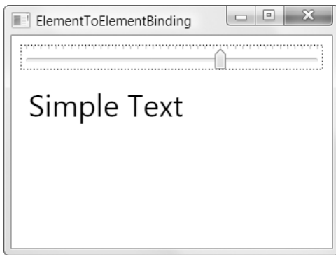
Figure 16-1. Linked controls through data binding
