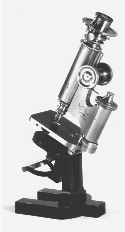
A 19th-century monocular microscope. These instruments were capable of high resolution but were difficult to use for extended periods of time. (Courtesy of Dr. Joseph Panno)
