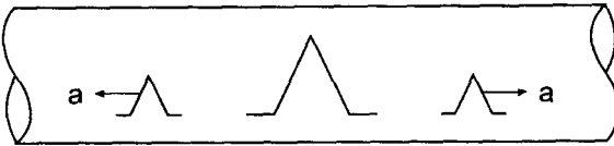
Figure 11.27 Acoustic wave propagation in an infinite duct.
