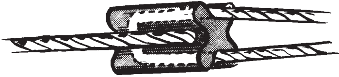
Figure 3-8. Strain insulator used for guy wires. Wires of insulator pull in opposite directions, resulting in compression.
