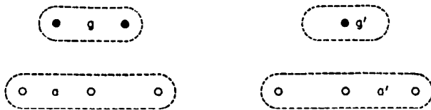
Fig. 24—Zero-sequence circuits formed by the 110 kv line (a), the 66 kv line (a'), the two ground wires (g), and the single ground wire (g').
