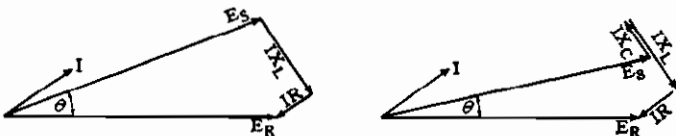
Fig. 33—When the load power factor is leading, a series capacitor is undesirable because it decreases the receiving end voltage.
