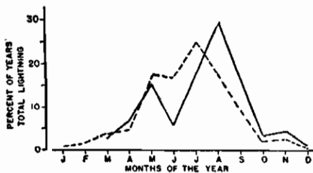
Fig. 26—Comparison between variance of disturbances on systems (solid curve) and monthly isokeraunic levels; McEachron and McMorris 46 .
