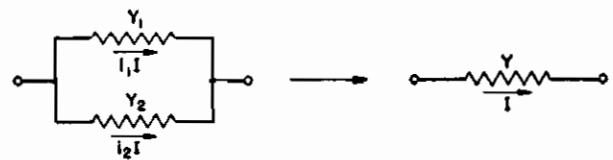
Fig. 22—Admittances in parallel.
