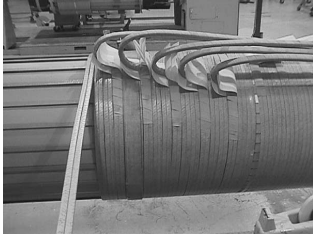
FIGURE 2.1.14 Layer windings (single layer with two strands wound in parallel).
