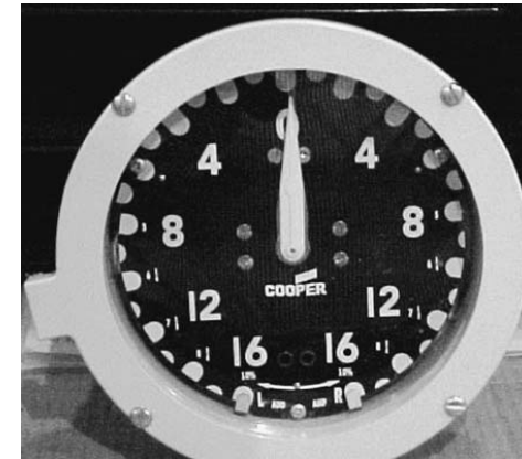
FIGURE 2.7.15 Tap-changer position indicator.
