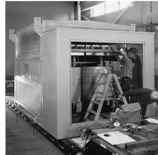
FIGURE 2.4.20 A 24-pulse dry-type transformer. 7000-kVA drive duty transformer, to be located in a tunnel, made of two 3500-kVA 12-pulse transformers. Each core and coil has 1100-V delta and wye secondary windings. Each core and coil has a 13,200-V extended-delta primary winding. One core and coil has its primary winding shifted -15°, while the other core and coil has its primary winding shifted +15°. One reconnectable primary spare core and coil can be used to replace either core and coil assembly. (Photo courtesy of Niagara Transformer Corp.)
