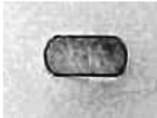
FIGURE 2.2.4 Cross section of enameled round wire after flattening. (By permission of ABB Inc., Jefferson City, MO.)
