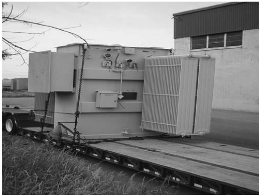
FIGURE 2.4.22 A 5000-kVA 18-pulse transformer ready for shipment. Motor drive duty, 13,800-V delta primary to secondaries of 1400-V delta, 1400-V delta +20°, and 1400-V delta -20°. (Photo courtesy of Niagara Transformer Corp.)
