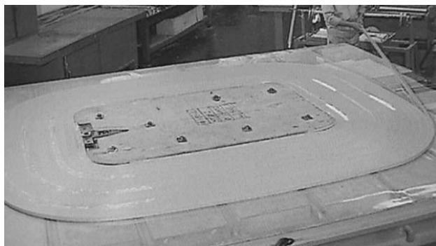
FIGURE 2.1.12 Pancake winding during winding process.
