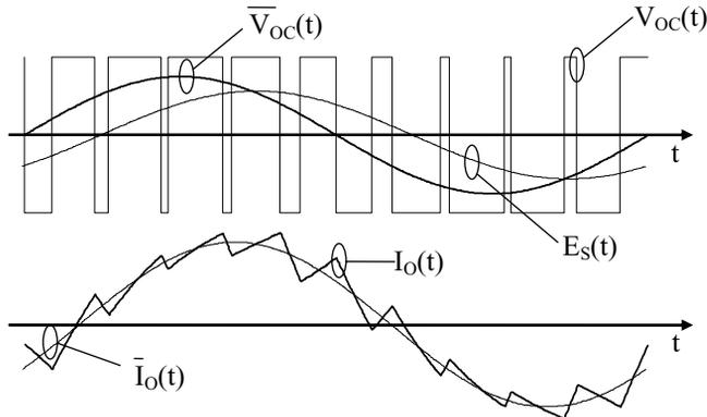
**FIGURE 2.4:** Example of PWM application to the VSI of Fig. 2.1. The instantaneous load voltage  $V_{OC}(t)$  is demodulated by the low-pass filter action of the inverter load. The resulting load current  $I_O(t)$  has an average value,  $\bar{I}_O(t)$ , whose waveform is determined by the instantaneous voltage average value  $\bar{V}_{OC}(t)$  (and by the load voltage  $E_S$ , here assumed to be sinusoidal).
