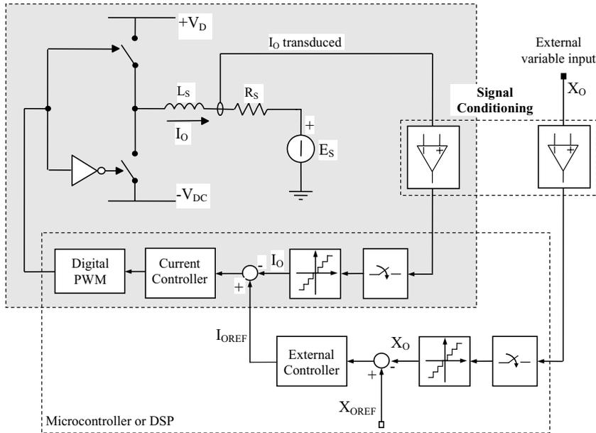
**FIGURE 5.1:** Typical organization of a multiloop digital controller.
