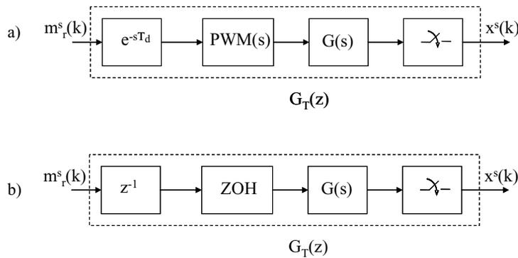
**FIGURE 3.14:** Equivalent dynamic model of computation delay, the PWM transfer function, the converter, and the sampler: (a) general form, (b) simplified representation, where the PWM is approximated as a zero-order hold (ZOH) and the control delay is equal to one modulation period.
