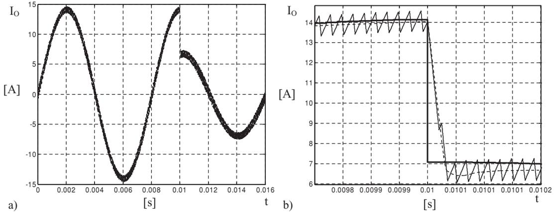
**FIGURE 3.11:** Simulation of the VSI with the controller designed according to the procedure reported in Aside 3. The depicted variable is the VSI output current  $I_o$ . (a) Controller response to a step reference amplitude change. (b) Details of the previous figure. It is possible to see that no calculation delay effect has been included in the simulation.
