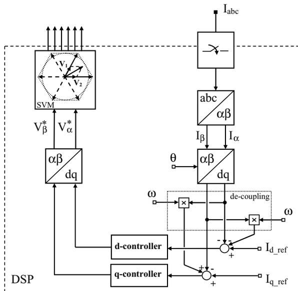
**FIGURE 4.8:** Organization of a three-phase digital current controller in the  $dq$  reference frame.
