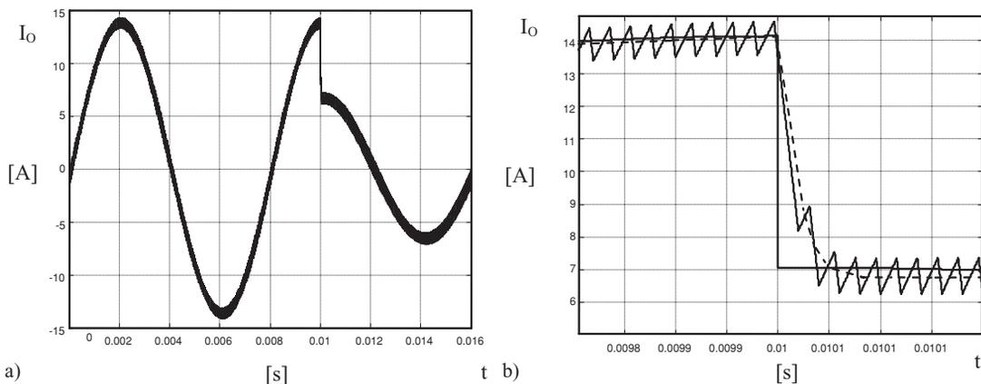
**FIGURE 2.11:** Simulation of the VSI depicted in Fig. 2.1 with the controller designed according to the procedure reported in Aside 2. The depicted variable is the VSI output current  $I_O$ . (a) Controller response to a step reference amplitude change. (b) Details of the previous figure.
