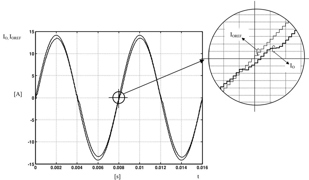
**FIGURE 3.21:** Simulation of the VSI with the predictive controller and dead-times. The dead-time effects are as follows: (i) crossover distortion, visible in the inset; (ii) steady-state error between the amplitude of the converter current and its reference. The sampled output current is shown instead of the instantaneous one to eliminate the ripple, which can mask the error. Dead-times are set to 5% of the modulation period, just to magnify the effect.
