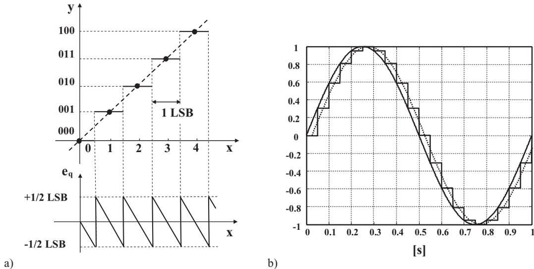
**FIGURE 3.3:** (a) Uniform quantizer transcharacteristic and quantization error  $e_q$ . (b) Sample and hold delay effect: compare the input signal (continuous line) and the reconstructed output signal, i.e., the fundamental harmonic component of the sampled signal (dotted line).
