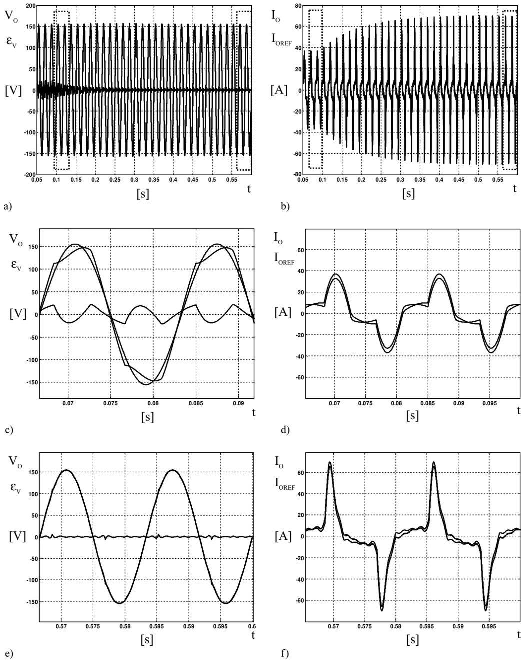
**FIGURE 5.17:** DFT filter based controller operation. (a) output voltage transient; (b) output current transient; (c) details of (a) before the repetitive controller is activated; (d) details of (b) before the repetitive controller is activated; (e) details of (a) after the steady state is reached with the DFT-based controller; (f) details of (b) after the steady state is reached with the DFT-based controller.
