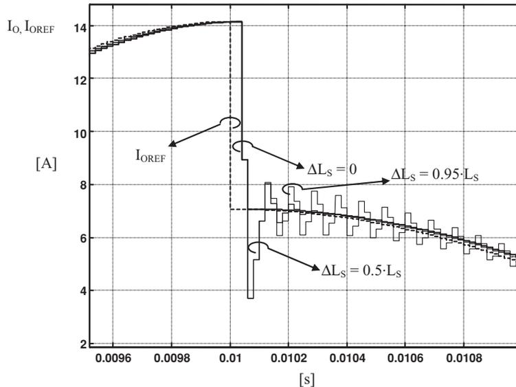
**FIGURE 3.19:** Simulation of the VSI with the predictive controller and different level of mismatch on parameter  $L_S$ . The figure shows the response to a step reference change of the sampled VSI output current  $I_O$ .
