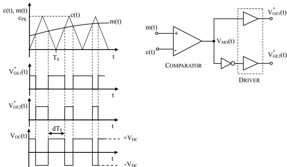
**FIGURE 2.3:** Analog implementation of a PWM modulator. The analog comparator determines the state of the switches by comparing the carrier signal  $c(t)$  and the modulating signal  $m(t)$ . The figure shows the logic state of each switch and the resulting inverter voltage. No dead-time is considered.
