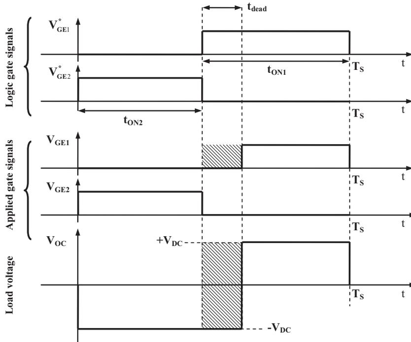
**FIGURE 2.2:** Dead-times effect: when a positive current  $I_O$  flows through the load, the actual on time for switch  $S_1$  is shorter than the desired one. Consequently, the average voltage across the load is different from the desired one.
