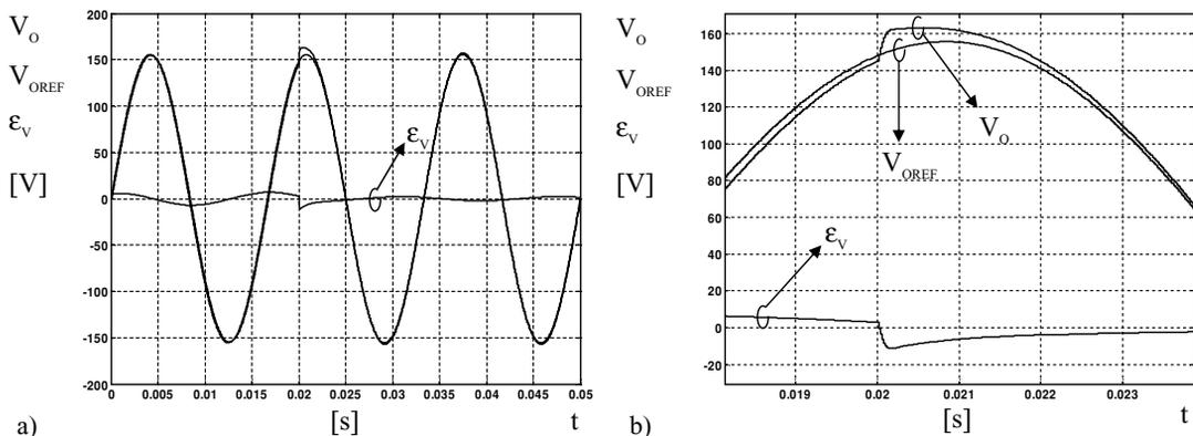
**FIGURE 5.6:** Dynamic response of the digital PI voltage controller: (a) response to a step load disconnection: the load current instantaneously reduces from about 9.1  $A_{RMS}$  to 0; (b) details of the previous figure.
