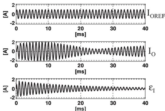
**FIGURE A8.1:** From top to bottom: current reference  $I_{OREF}$ , current  $I_O$ , and current error  $\varepsilon_1$  when the reference current is at  $k\omega_0$  and a resonant filter tuned at harmonic  $k$  is used.
