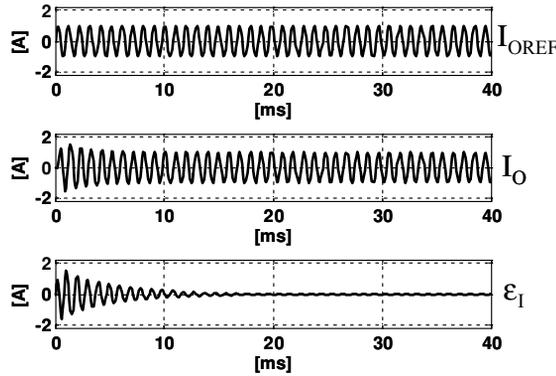
**FIGURE A8.3:** From top to bottom: current reference  $I_{OREF}$ , current  $I_O$ , and current error  $\epsilon_I$  when the reference current is at  $k\omega_0$  and a resonant filter tuned with lead angle  $\phi_k$  at harmonic  $k$  is used.
