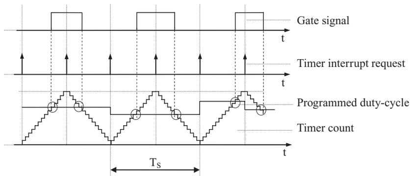
**FIGURE 2.7:** Double update mode of operation for a digital pulse width modulator. Duty-cycle update is allowed at the beginning and at a half of the modulation period. Note that the gate pulses are now symmetrically allocated within the modulation period (in steady state).
