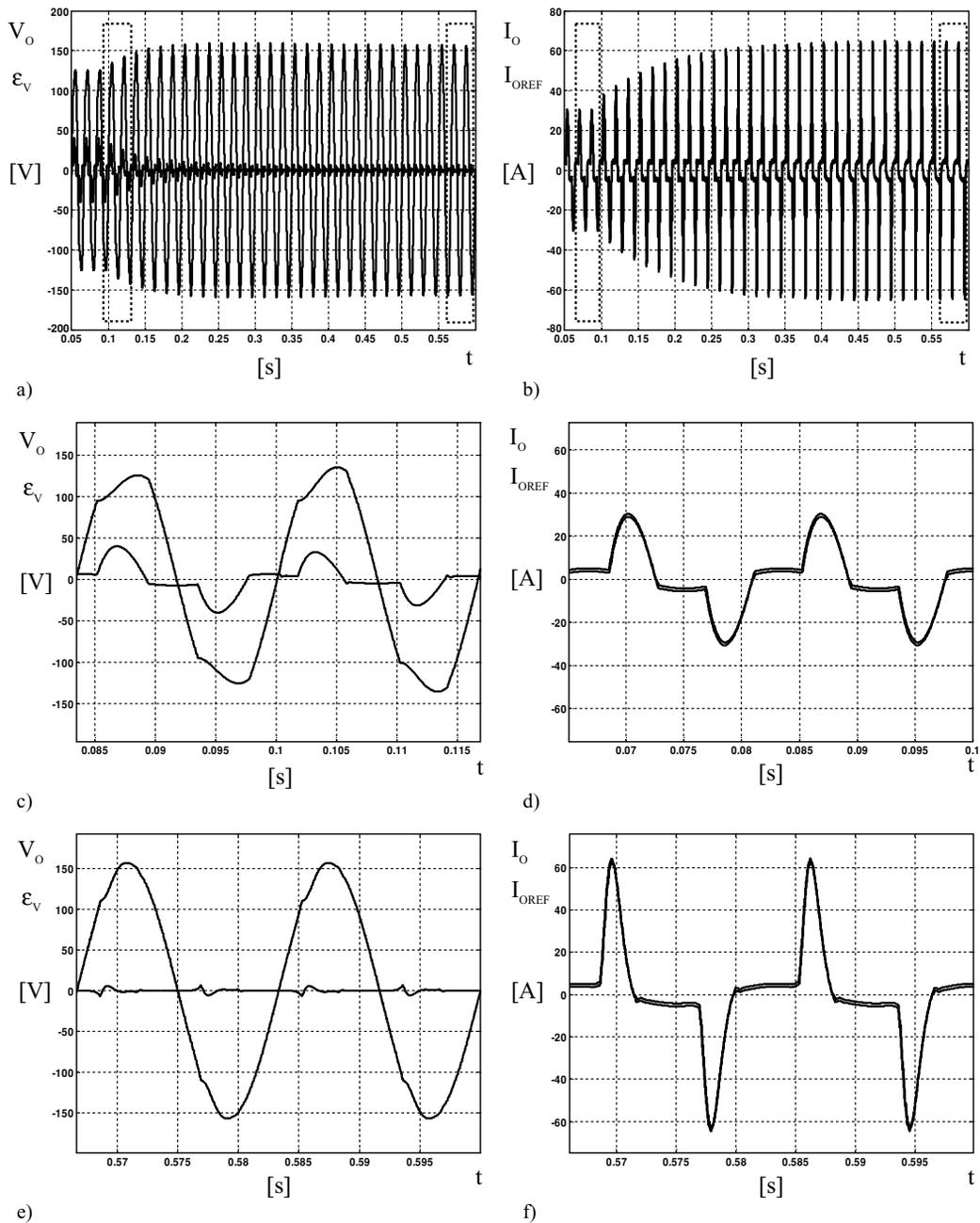
**FIGURE 5.14:** Repetitive-based controller operation. (a) output voltage transient; (b) output current transient; (c) details of (a) before the repetitive controller is activated; (d) details of (b) before the repetitive controller is activated; (e) details of (a) after the steady state is reached with the repetitive controller; (f) details of (b) after the steady state is reached with the repetitive controller.
