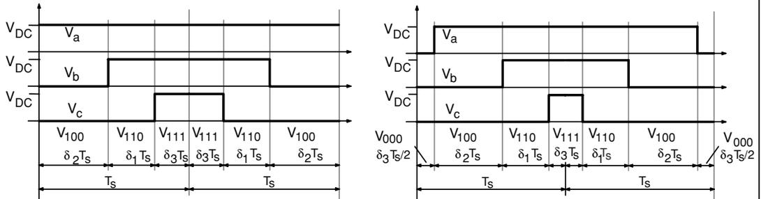
**FIGURE A6.3:** Two different application sequences for the same output voltage vectors. The sequence on the left implies a minimization of the number of switchings. The sequence on the right implies the minimization of the current ripple amplitude (voltage pulses have even symmetry). Note that each strategy develops in two adjacent modulation periods.
