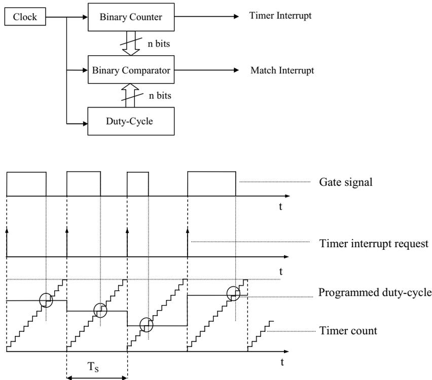
**FIGURE 2.5:** Simplified organization of a digital pulse width modulator. The binary comparator triggers an interrupt request for the microprocessor any time the binary counter value is equal to the programmed duty-cycle (match condition). At the beginning of the counting period, the gate signal is set to high and goes low at the match condition occurrence.
