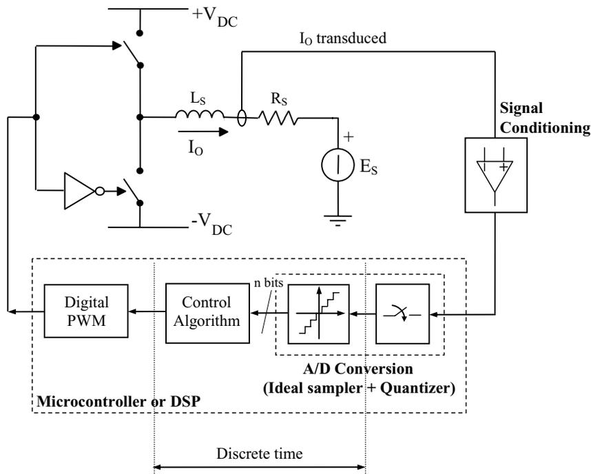
**FIGURE 3.1:** Typical organization of a digital current controller.
