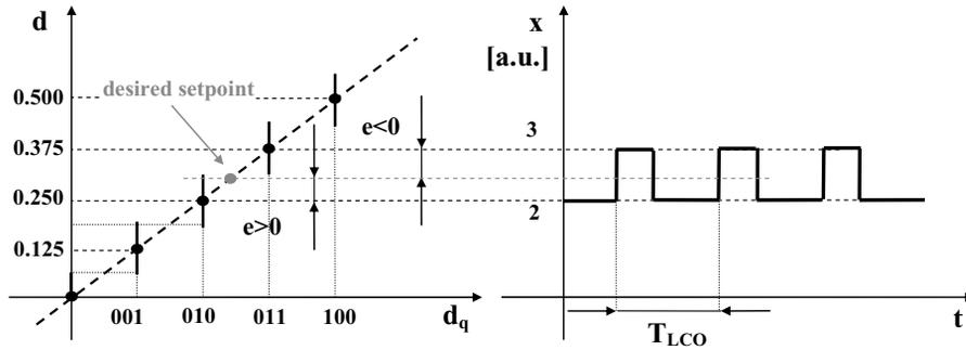
**FIGURE 3.5:** Example of limit cycle occurrence. The desired set-point for the output control variable  $d$  is not one of the possible output values. Consequently, the system oscillates, with period  $T_{LCO}$ , between the two closest outputs. Here we assume that the system includes at least one integral action in the transfer function from the input to the output.
