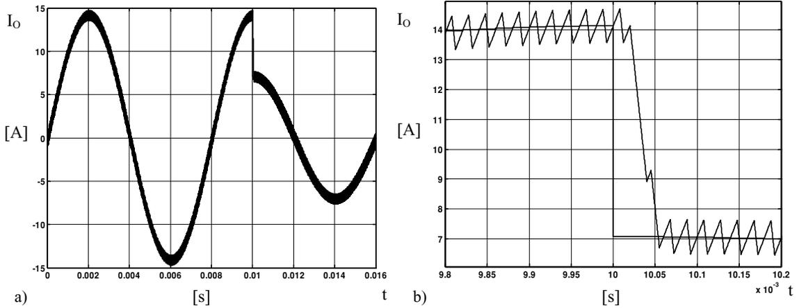
**FIGURE 3.18:** Simulation of the VSI with the predictive controller. The depicted variable is the VSI output current  $I_O$ . (a) Controller response to a step reference amplitude change. (b) Details of the previous figure.
