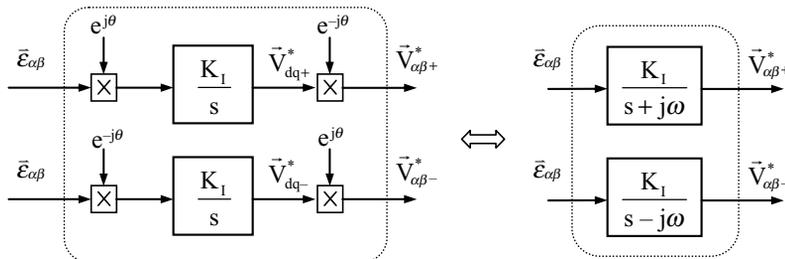
**FIGURE 4.11:** Laplace transformation of the rotating reference controller.
