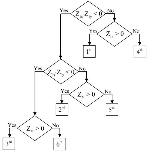
**FIGURE A6.2:** Flow chart of the sector identification algorithm.
