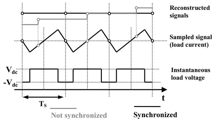
**FIGURE 3.4:** Example of synchronized sampling and switching processes. In case the sampling takes place always at the beginning (or in the middle) of the modulation period, the average current value is automatically obtained. If the sampling frequency is lower than the switching one, an aliased, low-frequency component appears on the reconstructed signal.
