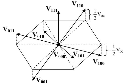
**FIGURE 4.5:** Tridimensional view of the space vector hexagon.
