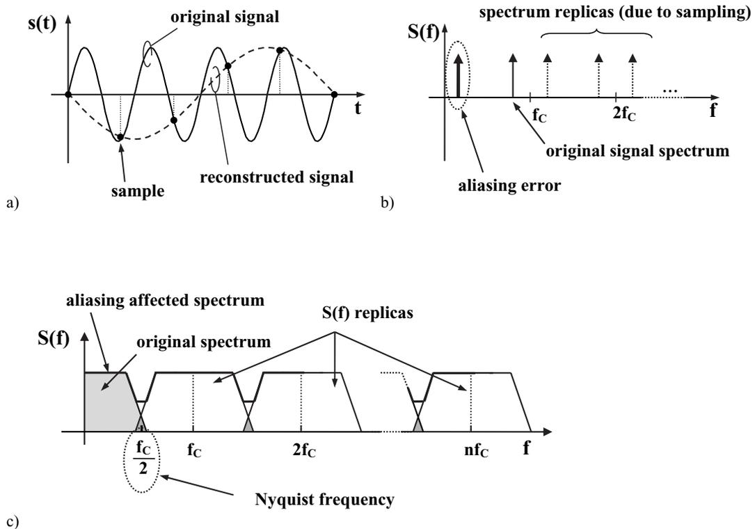
**FIGURE 3.2:** (a) Effect of a too low sampling frequency on the reconstructed signal (aliasing). (b) Interpretation of the aliasing effect of (a) in the frequency domain. Note how a low-frequency spectrum component is generated because of aliasing. (c) A more general situation: a distorted, aliasing-affected, spectrum is reconstructed because of the partial overlap of spectrum replicas.
