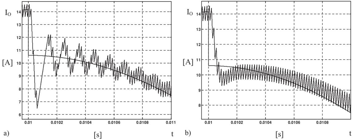
**FIGURE 3.12:** Simulation of the VSI with the digital PI controller including the calculation delay. (a) Details of the controller response to a step reference amplitude change without redesign: undershoot and oscillating response. (b) Details of controller response with redesign: reduced undershoot, reduced speed of response, increase of phase shift.
